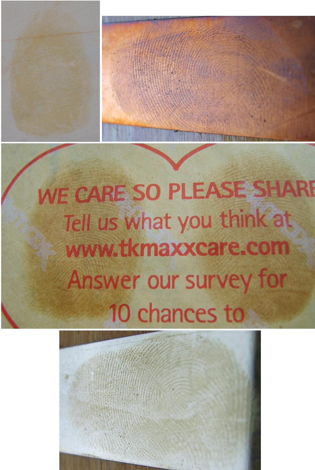
Figure 92: Fingerprints developed using Cobalt-Rubeanic acid method on glass (top left), copper (top right), thermal paper (middle) and stainless steel (bottom)
