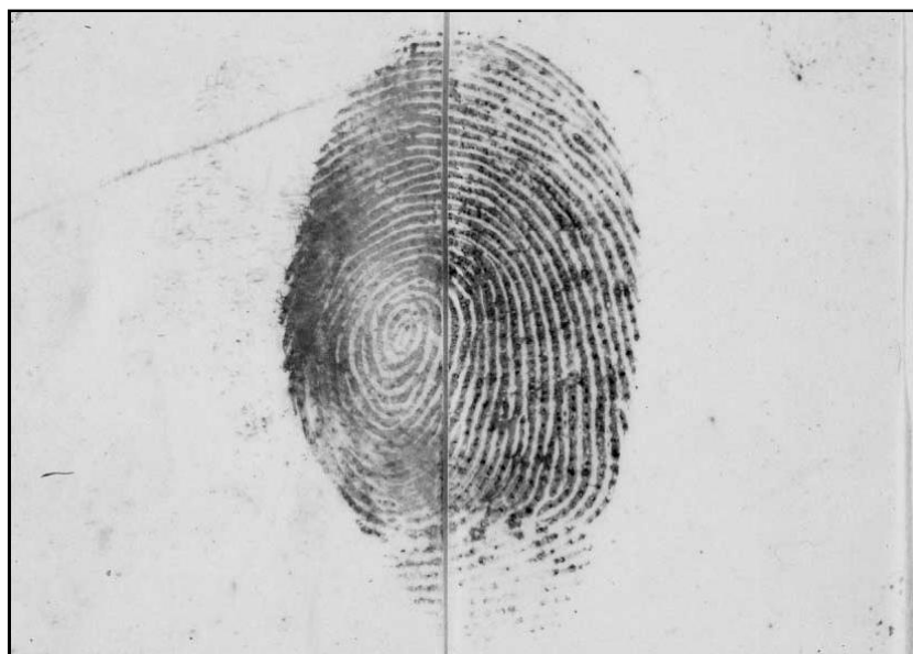
Figure 12: Example of finger-mark developed on a porous surface (white paper) using the old method (left) against the proposed optimized method (right) 26
