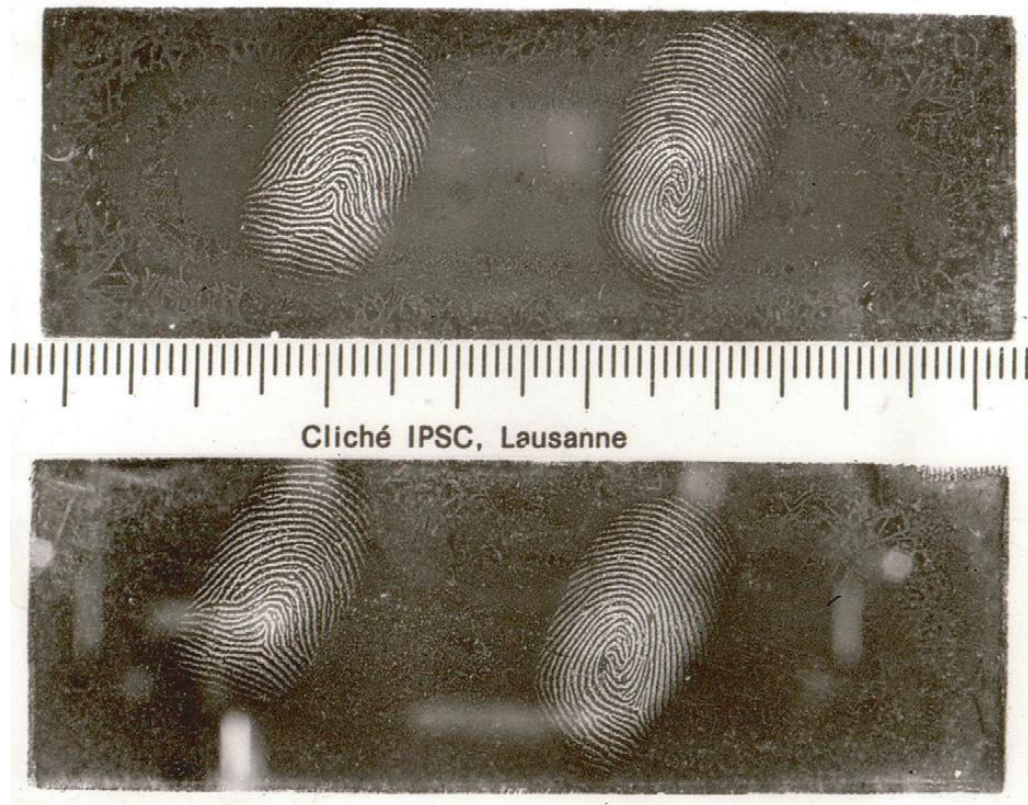
Figure 18: 3 year-old latent finger-marks on glass after treatment by VMD (negative prints) 44
