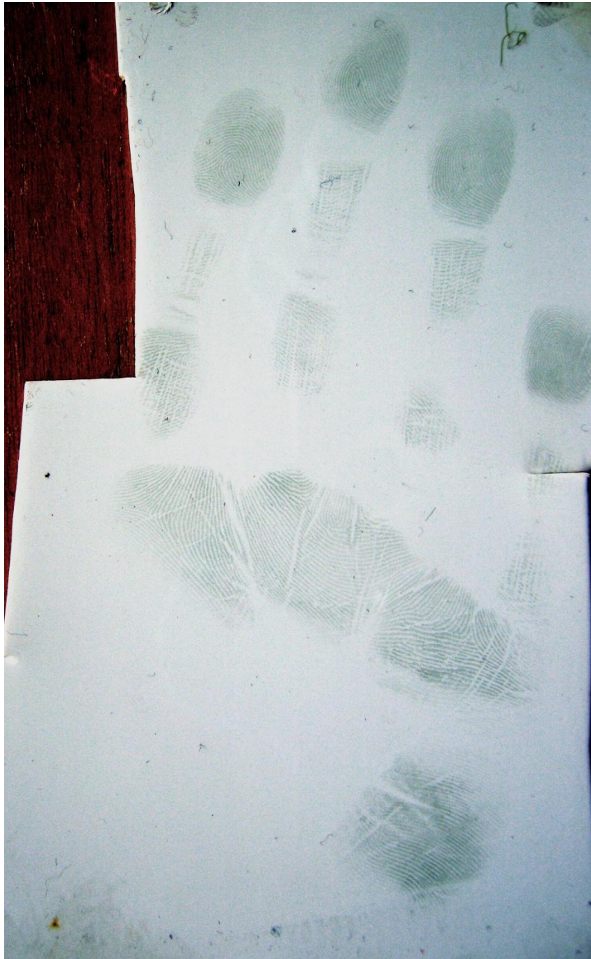
Figure 101: Palm print developed with rubeanic acid after holding an old copper pipe for 30 seconds
