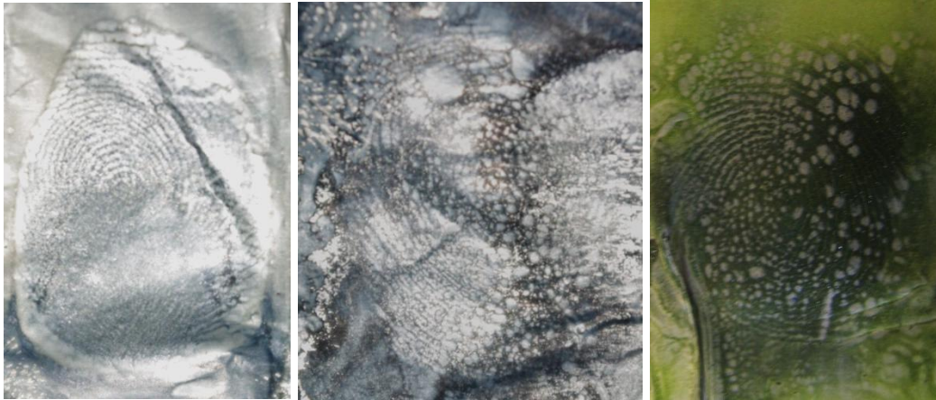
Figure 75: A set of developed fingerprints on aluminium foil using 10% PMA solution with 1 short spray (left), 2 short sprays (middle), excessive spray (right)
