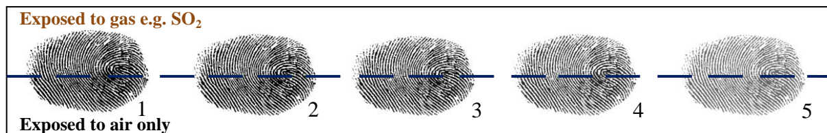
Figure 53: Illustration of how the direct comparison of fingerprints is undertaken for the ESDA process
