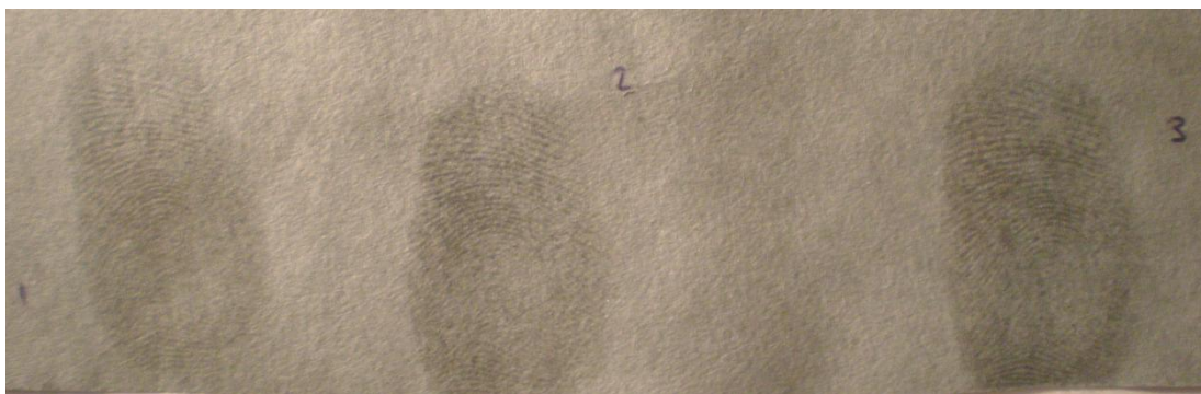
Figure 89: Developed fingerprints on filter paper using 0.15% ethanolic rubeanic acid
