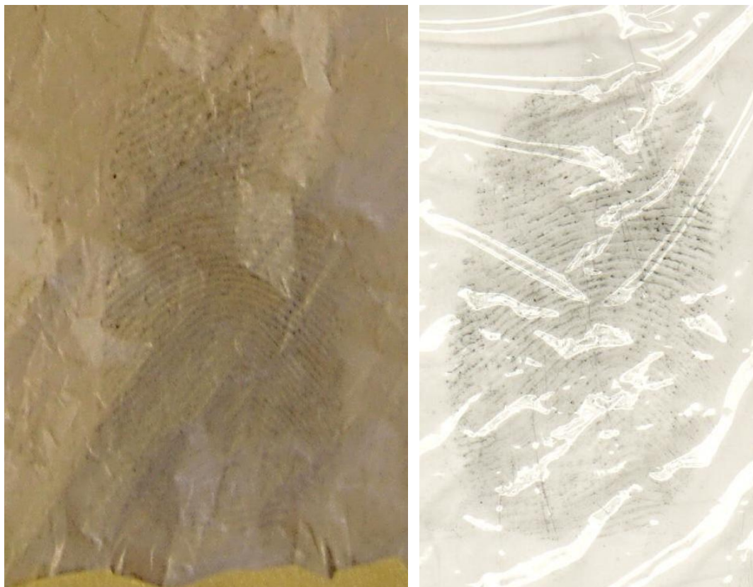
Figure 84: Prints developed on a white carrier bag (left) and Clingfilm (right) using the optimized method
