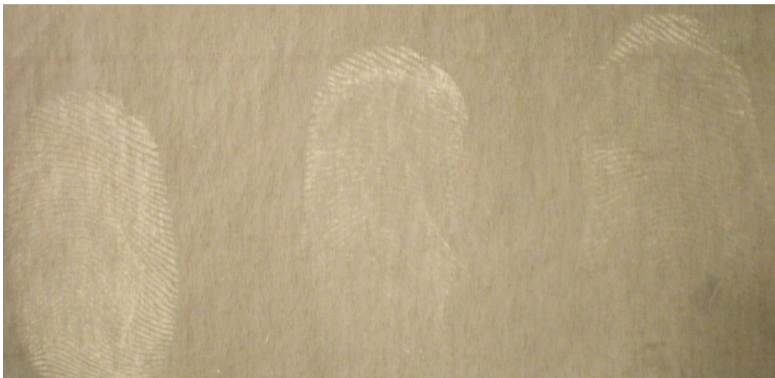
Figure 94: 2 month old fingerprints on filter paper developed using the optimized copper-rubeanic acid method
