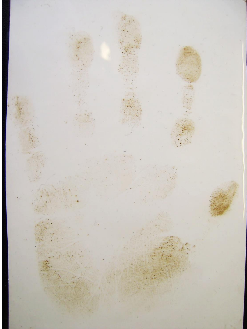
Figure 102: Palm print developed with rubeanic acid after contact with lead for 30 minutes
