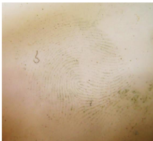
Figure 100: Grade 4 fingerprint developed on a gel lifter with rubeanic acid after touching a copper plate for 30 seconds
