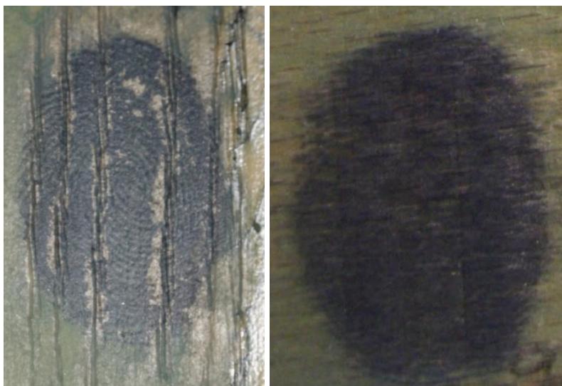
Figure 72: Fresh fingerprints developed at 100°C using 10% PMA solution on laminated wood (left) and raw wood (right)
