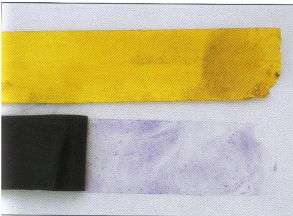
Figure 13: Gentian violet on yellow adhesive tape and transferred from black adhesive tape 24
