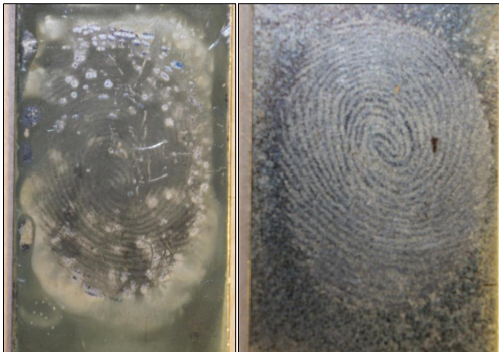
Figure 76: Developed fingerprints on steel using 10% PMA solution with excessive spray (left) and 1 short spray (right)
