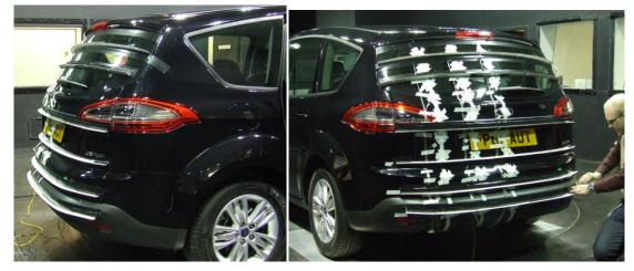
Figure 7.3- Full scale test vehicle shown in configuration 1 with pressure 'spades' attached to one half of the vehicle base surface
