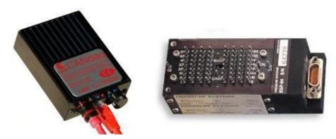
Figure 2.3 - Pressure scanner and CanDaq
