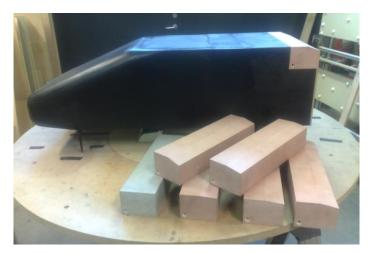
Figure 3.2 - Windsor model and interchangeable rear chamfer components
