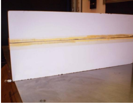
Figure 4.9: A plate was used for horizontal plane alignment
