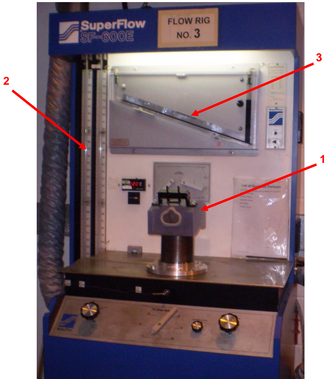
Figure 4.3: SuperFlow SF600E. 1-Cylinder head being tested, 2-Pressure manometer, 3- Percentage flow manometer
