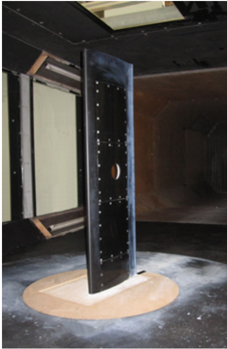
Fig. 1 Three dimensional model installed in Loughborough University’s Large Wind Tunnel (lower surface shown)
