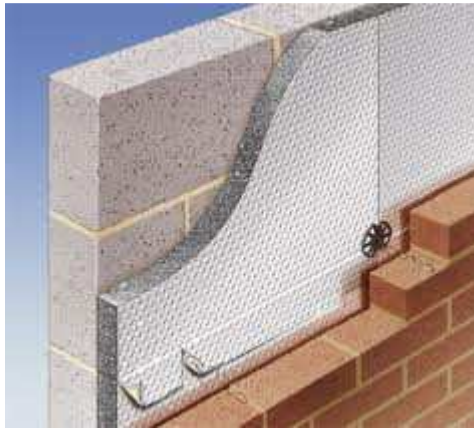
Figure 2-6. Schematic of cavity wall construction
