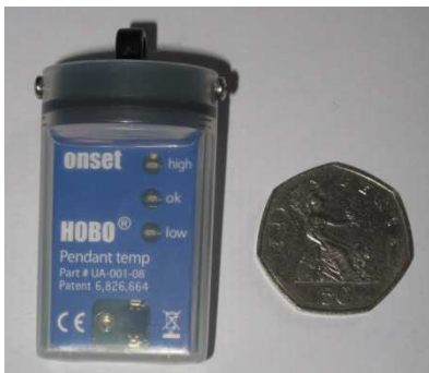
Figure 3-3. Hobo data logger used to measure internal air temperature in 292 dwellings in Leicester City.
