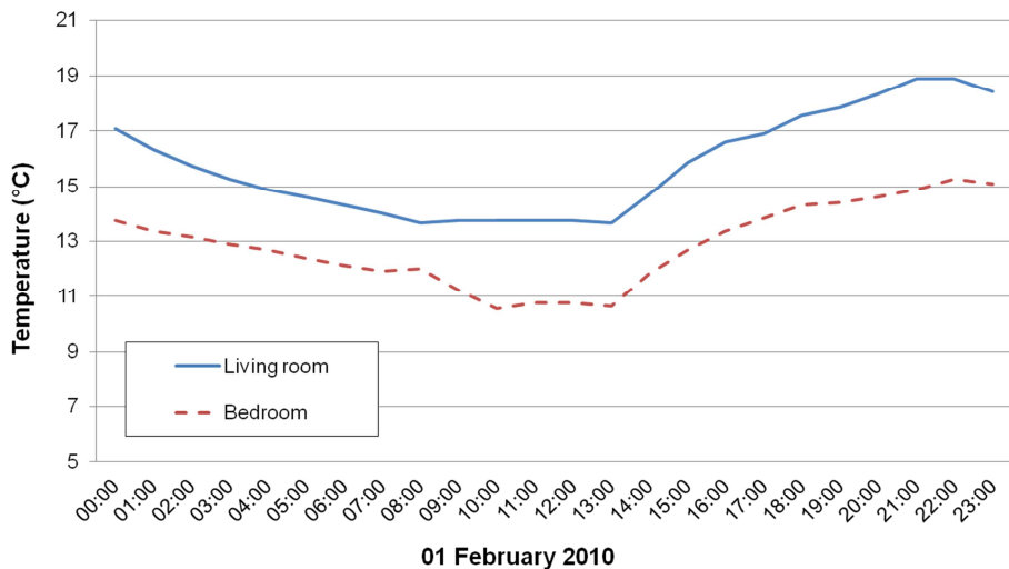
Figure 3-21. Example of temperatures where thermostatic control cannot be observed from the temperature traces measured in on 1 st February 2010.
