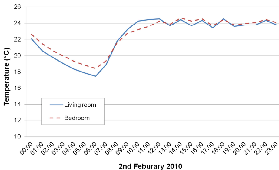
Figure 3-20. Temperature plot of a single day in one dwelling showing a single heating period and successful thermostatic control.
