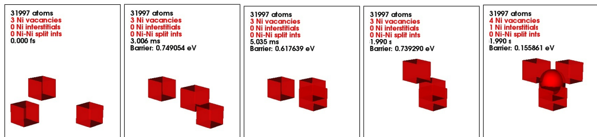
Figure 5.23: Snapshots of the steps involved in transformation of 3 vacancies into 3 vacancies SFT, associated energy barriers are shown at each snapshot.
