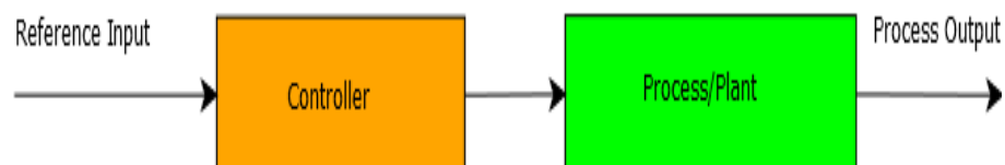
FIGURE 3-5: Open Loop Control Action
