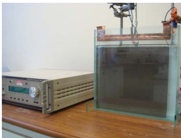
Figure 3.8. Image showing a one compartment electrochemical tank used for all large-scale experiments. The tank dimensions were 35 x 35 x 5 cm.
