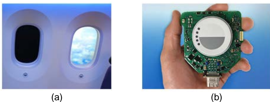
Figure 2.6. (a) EC windows installed in the new Boeing Dreamliner. (b) A window-seat controller which allows the passenger to activate the system and change the amount of visible light entering the cabin. 95
