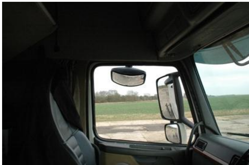
Figure 1. Image of the approximate view afforded to the driver of a VOLVO FH Category N 3 vehicle
