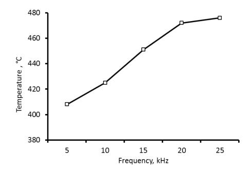
Figure 6-12: Temperature of process zone at various frequencies of vibration
