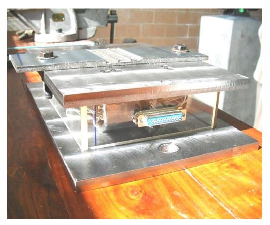
Figure 2-16: Three component dynamometer with hexagonal transducer [75, 81, 82]
