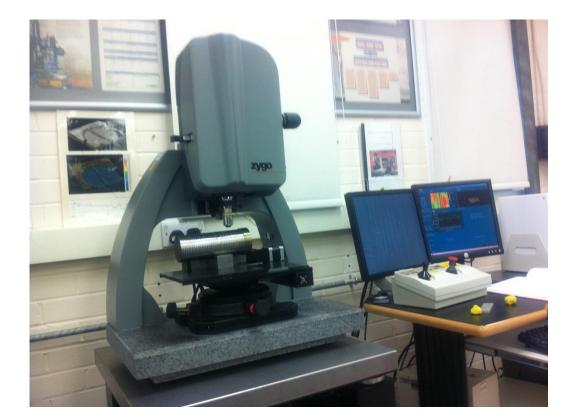
Figure 4-25: Experimental setup for surface roughness analysis using Zygo<sup>®</sup> interferometry
