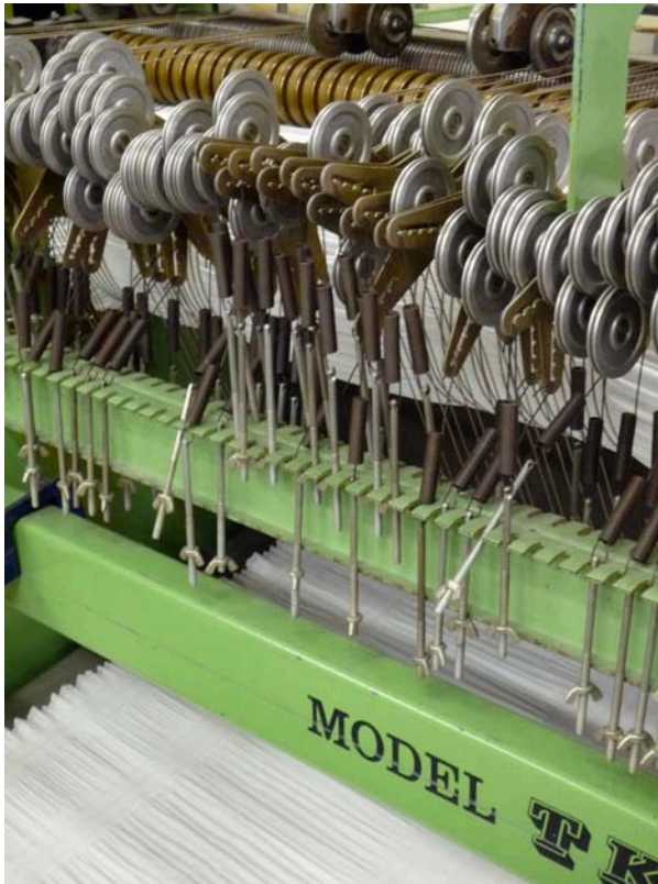
Left: Figure 5: Inoue Pleats Co. Ltd (2008). Automated princess pleating machine. Photograph: Rachel Philpott. © Rachel Philpott.
