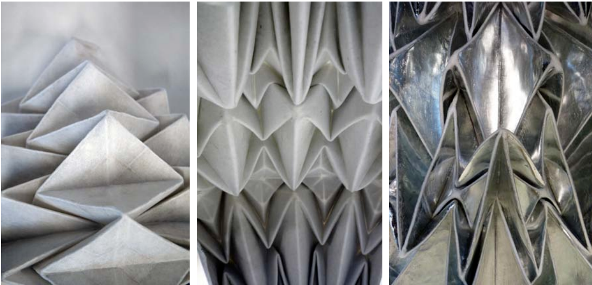
Left, Right and Centre: Figures 9a, 9b and 9c: Rachel Philpott (2010). Deployable textile structures with shape-memory, composite materials formed using laser cutting and hand making techniques. Photograph: Rachel Philpott. © Rachel Philpott.
