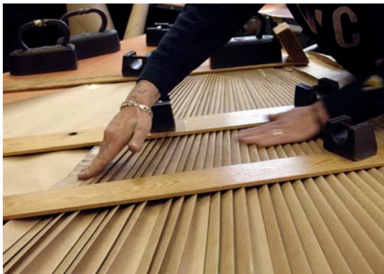
Left: Figure 7: F. Ciment (Pleating) Ltd (2005). Worker hand pleating textiles using card moulds. Photograph: Rachel Philpott. © Rachel Philpott.
