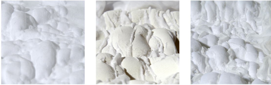
Left- Figure 6: Cotton/lycra mistakenly silk-screen printed with flocking adhesive. Middle- Figure 7: Cotton/lycra silk-screen printed with puff binder. Right- Figure 8: Cotton/lycra and silk mousaline layered fabric, silk-screen printed with flocking adhesive and flocked.
