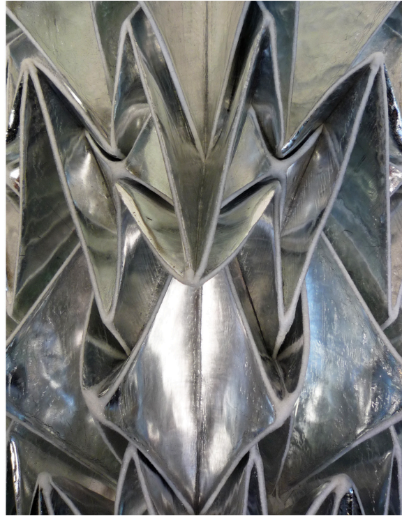
Left- Figure 4: Deployable textile with shape-memory, form improvised after an error discovered in making process. Right- Figure 5: Foil-finished deployable textile with shape-memory, made to original folding pattern.
