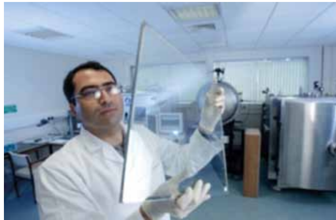
Figure 3: Fabricated vacuum glazing
