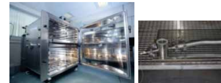
Figure 2: Vacuum oven and pump-out system
