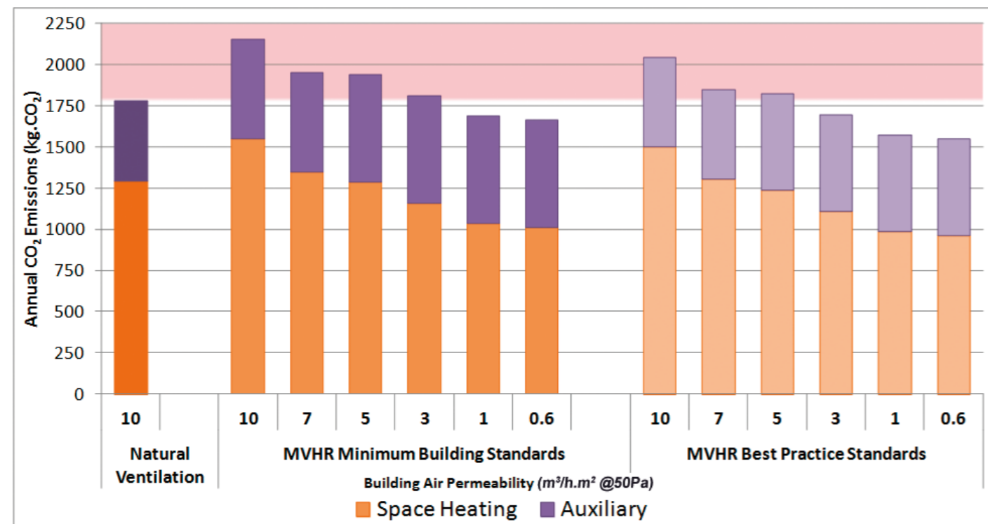
Figure 3: Modelled annual space heating and auxiliary CO 2 emissions of the E.ON Retrofit Test House
