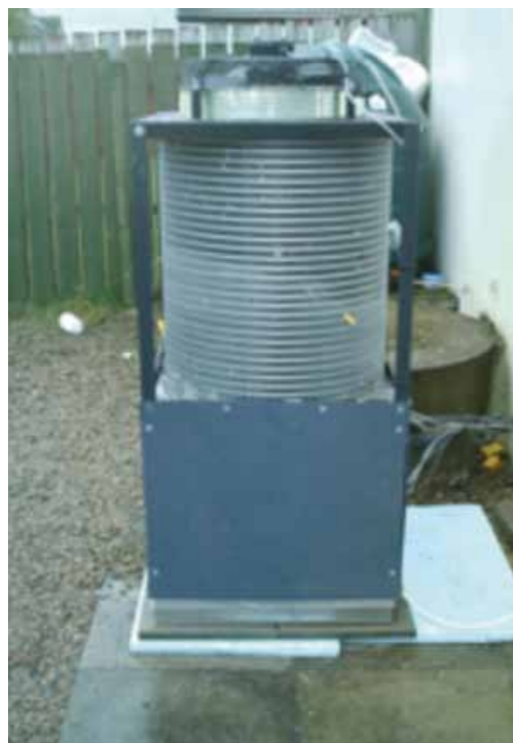
Figure 2: Prototype of CALEBRE electric EVI heat pump (developed at Ulster University)
