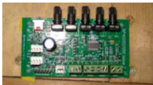
Figure 4: New controls to allow independent fan speeds for better system balancing supplied by the MVHR manufacturer
