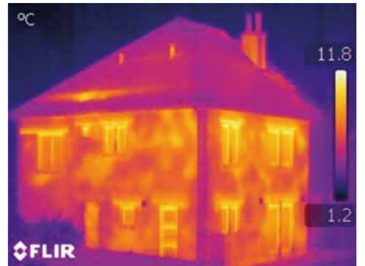
Figure 5: Thermal image of the CEH E.ON Research House after the retrofit of insulation
