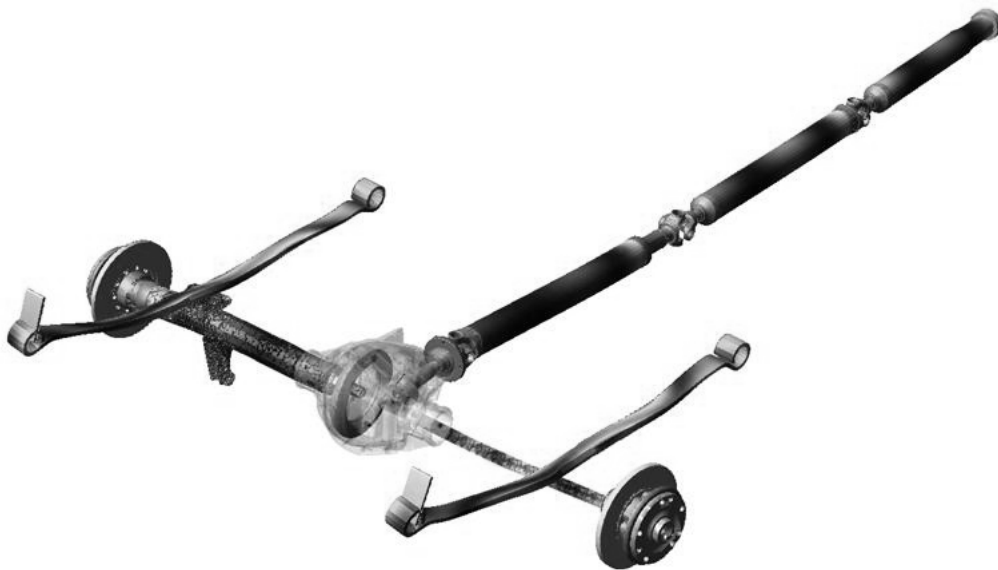
Figure 8: The drivetrain model: Wind-down mode of leaf springs with untwist of the rear axle (509 Hz)
