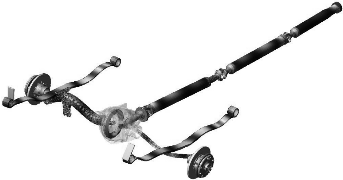
Figure 11: The drivetrain model: Butterfly mode of the rear axle with multiple leaf spring bending (772 Hz)
