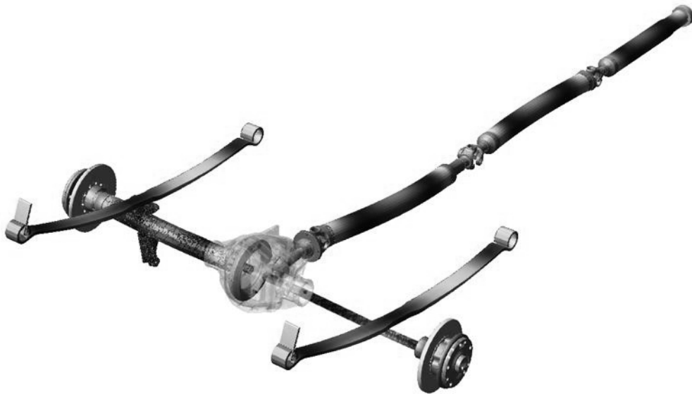
Figure 10: The drivetrain model: Lateral sway mode of the driveline and rear axle which may induce wheel tramp (240 Hz)
