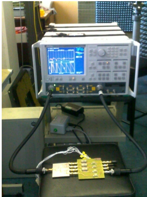
Figure 6-24: Feed network characteristics measurement.
