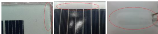
Fig. 3 Defects observed after damp heat testing: edge/corner delamination (a), moisture ingress (b) and bubble near electrode exit (c)
