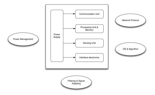
Figure 2-2 Sensor node functional components (Benini et al., 2006)
