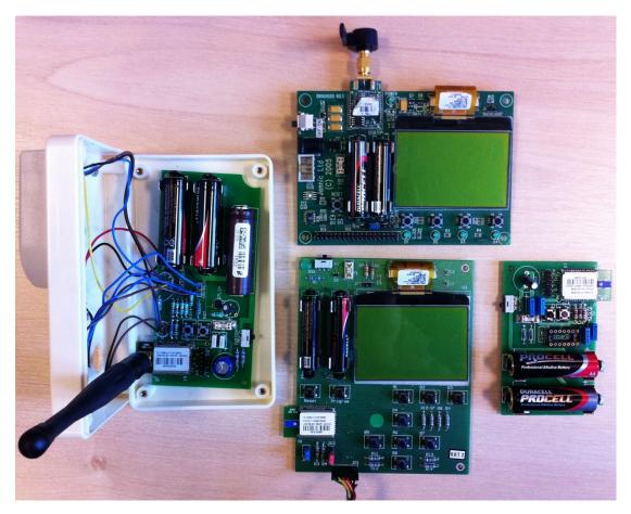
Figure 5-7 Jennic development kit (up: Coordinator, down: SSP Router, left: end device with illumination sensor, right, end device with temp sensor)
