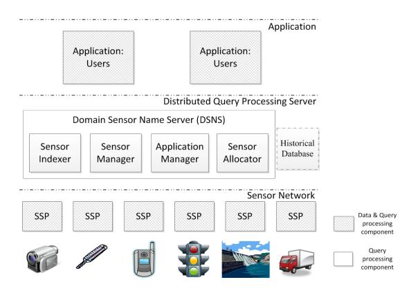
Figure 5-1 Distributed FSN architecture (Xu and Yang, 2010)
