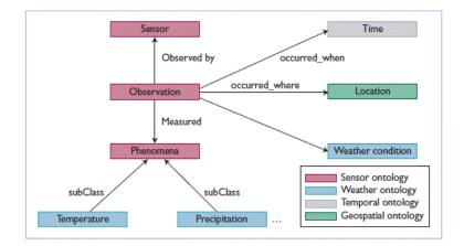
Figure 4-3 Concepts and relations in Semantic Sensor Web (Shethet al., 2008)
