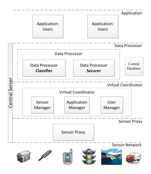
Figure 4-4 System architecture of centralized Federated Sensor Network (Xu and Yang, 2009)
