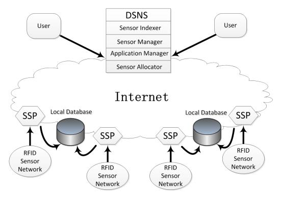
Figure 8-2 IoT service-oriented architecture for supply chain management
