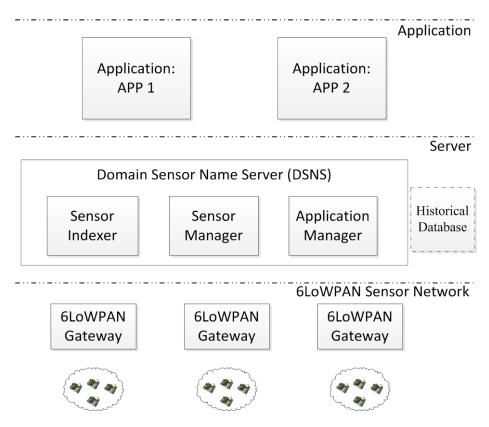
Figure 6-1 6LoWPAN Federated Sensor Network architecture
