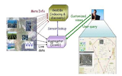
Figure 4-2 SenseWeb Architecture (Santanche et al., 2005)
