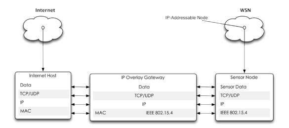
Figure 3-5 IP overlay network solution
