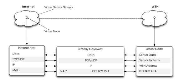
Figure 3-6 Overlay sensor network solution
