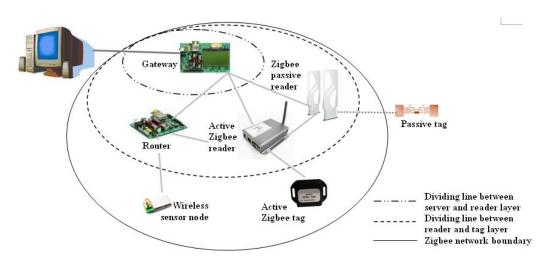
Figure 8-1 Hybrid RFID sensor network architecture (Yang et al., 2011)
