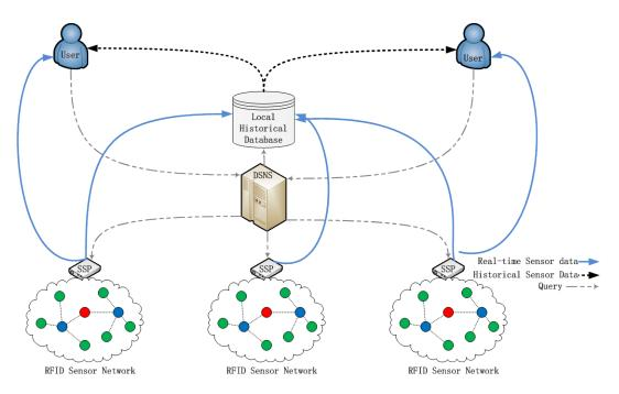
Figure 8-3 Dataflow of the IoT architecture for supply chain management
