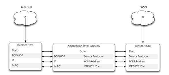
Figure 3-3 Application-level gateway solution
