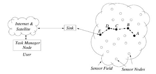
Figure 1-1 Sensor nodes scattered in a sensor field (Akyildiz et al., 2002)
