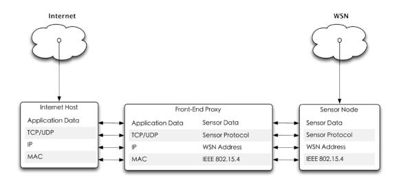
Figure 3-2 Front-end Proxy solution
