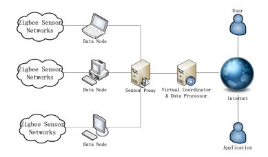
Figure 4-5 Demonstration architecture of centralized Federated Sensor Network
