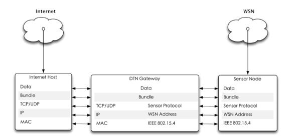
Figure 3-4 DTN gateway solution
