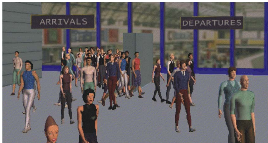
Figure 3.9 Simulation of human movement at a train station using a rule based behavioural system (Schweiss et al. 1999)
