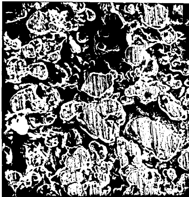
Fig. 29 a S.E.M Photographs for Surfaces of Calcium Stearate Specimens Densities: 1) 5.55 ; 2) 5.93 ; 3) 6.3; 4) 6.5 ; 5) 6.8 \text{g/cm}^3 .
