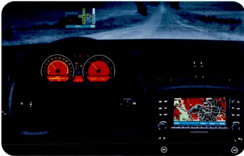
Figure 2.19. An automotive Head Up Display showing direction of turn information produced by Seimens and implemented in BMW 5 and 6 series vehicles
