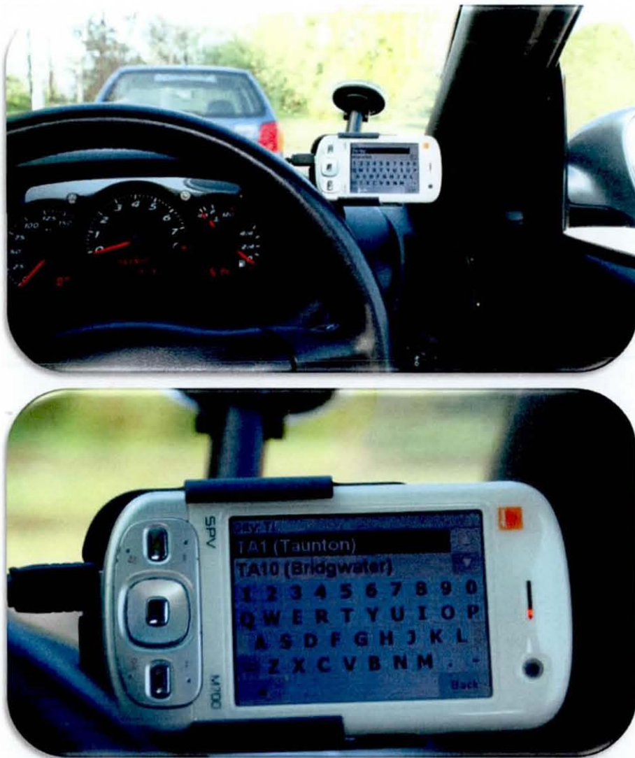
Figure 8.17. An example of the on screen keyboard used in current portable navigation system (example shown Tomtom v6 running a Windows based smartphone with 3.5 inch screen)
