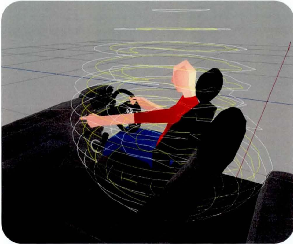
Figure 4.13: The analysis environment in the human modelling system SAMMIE, showing the postures adopted and the reach contours that are used to assess the reach-ability of various locations
