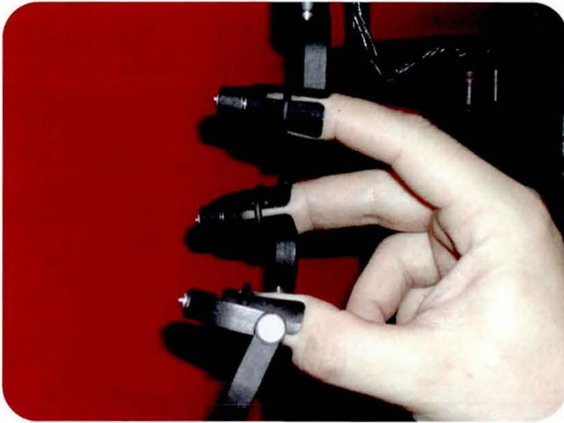
Figure 2.12. The device used in the McKnight study examining the use of three combined Phantom interfaces to provide three finger haptic feedback for virtual object exploration
