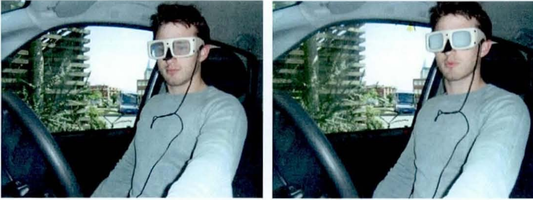
Figure 2.3: The use of Occlusion glasses in the automotive environment
