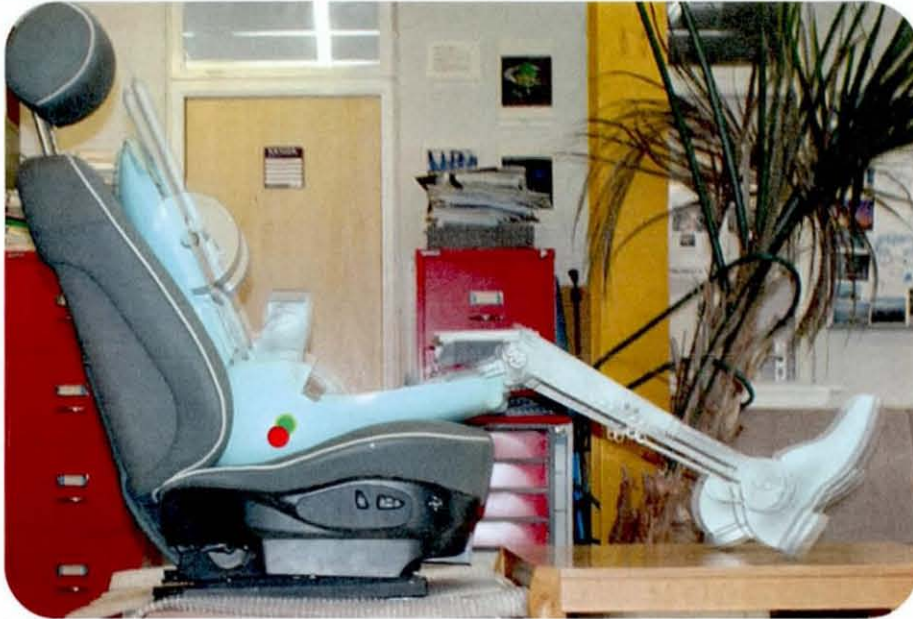
Figure 4.12: The SAE H-Point Manikin shown with a loaded condition superimposed over an unloaded condition. The green and red dots show the change in the Hip point due to seat compression under load
