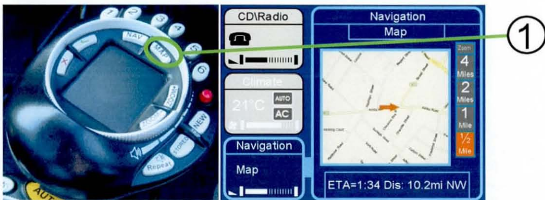
Figure 7.2. The control that is used to select a map view in the navigation system on the PTI
