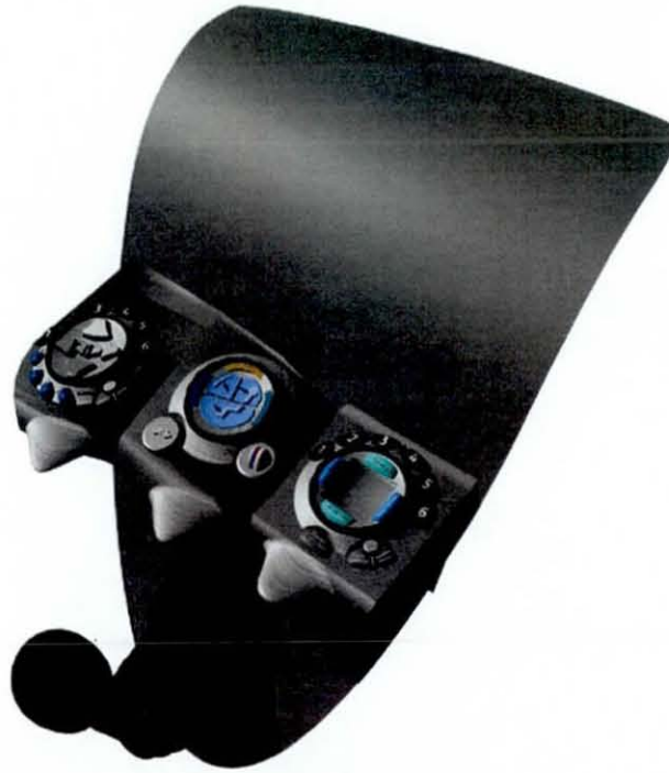
Figure 5.13: The design of a mounting structure that improved the reach-ability of the dashboard within the Honda Civic
