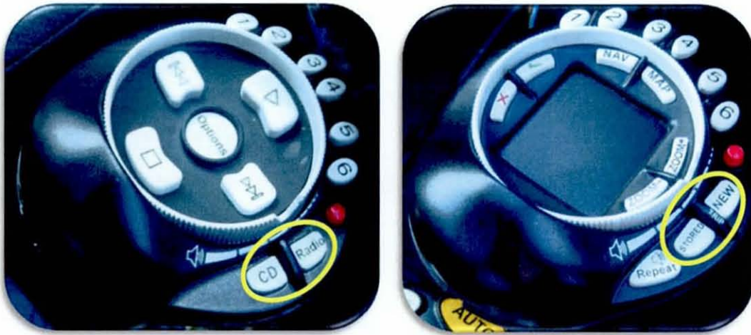
Figure 8.4. Two sets of controls that were not used non-visually
