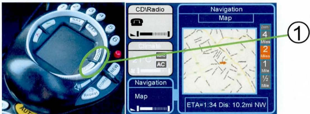
Figure 7.5. The task stages used to change the zoom level of the map view on the PTI system
