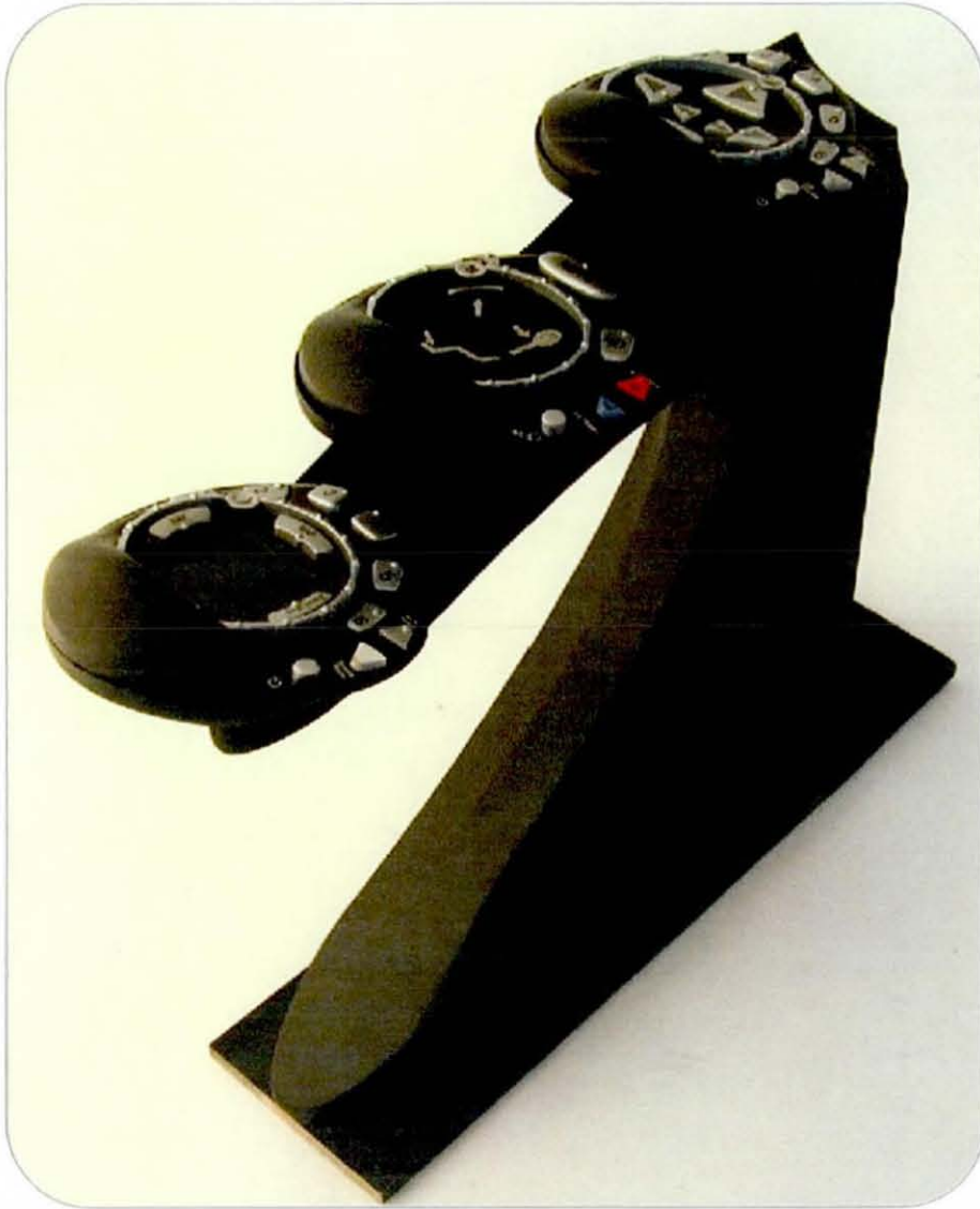
Figure 5.31 The PTI that was used during the simulator study, manufactured using SLA rapid prototyping technology, with tactile feedback for button depression detection
