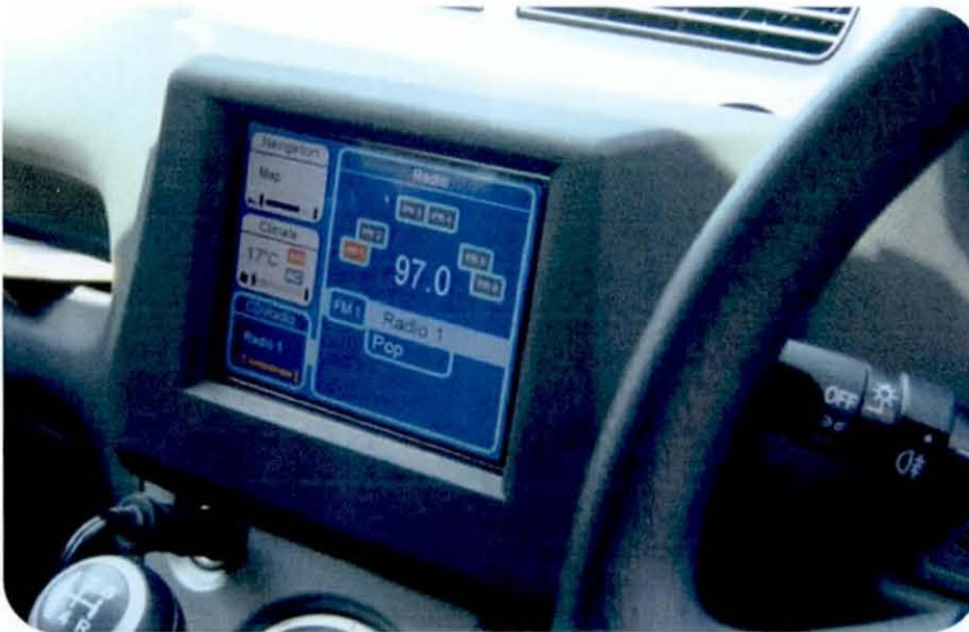
Figure 5.52. The final PTI software running on a 10 inch screen with a custom screen surround
