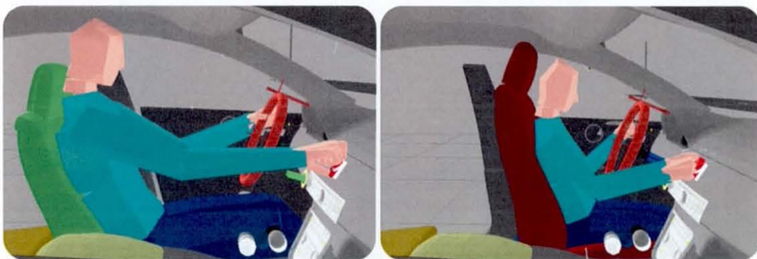
Figure 4.6: The range of virtual human model sizes used to evaluate the adjustability ranges of a new road vehicle
