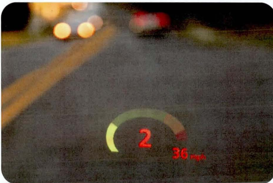
Figure 2.18. An automotive Head Up Display implemented in a 2007 BMW M5
