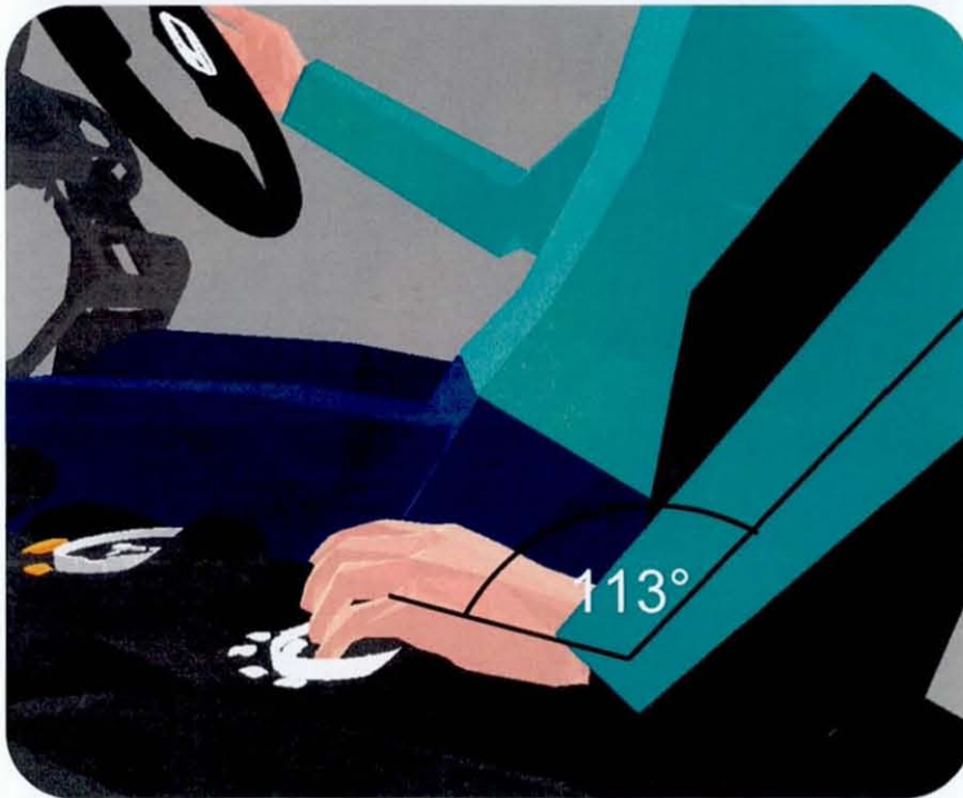
5.27. The improvement in wrist angle that is allowed by angling the arrays (top image, flat arrays. Bottom image, angled arrays)
