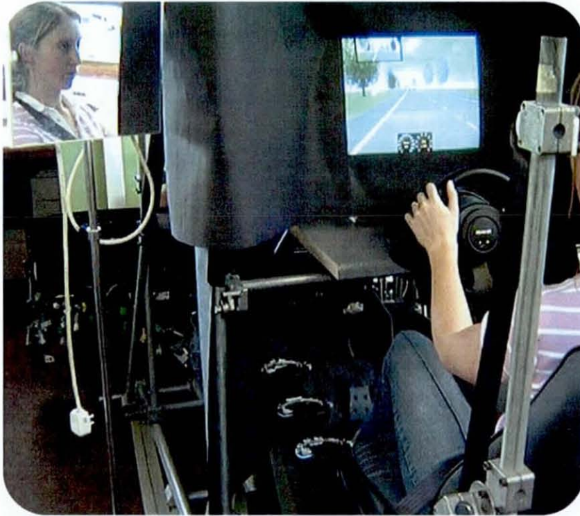
Figure 5.34. The simulator experimental setup using a mirror to capture glance durations
