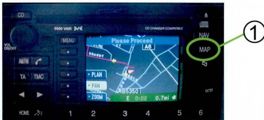
Figure 7.1. The control that is used to select a map view in the navigation system of the baseline interface
