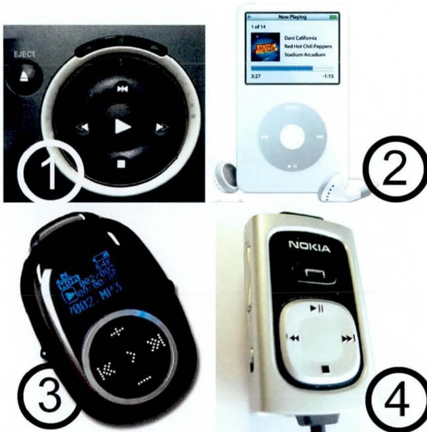
Figure 5.3. Arrangement of the play, stop, skip forward and skip back controls for a range of products. 1: Video cassette recorder controls. 2: I-pod controls. 3: Mp3 player controls. 4 Remote control.
