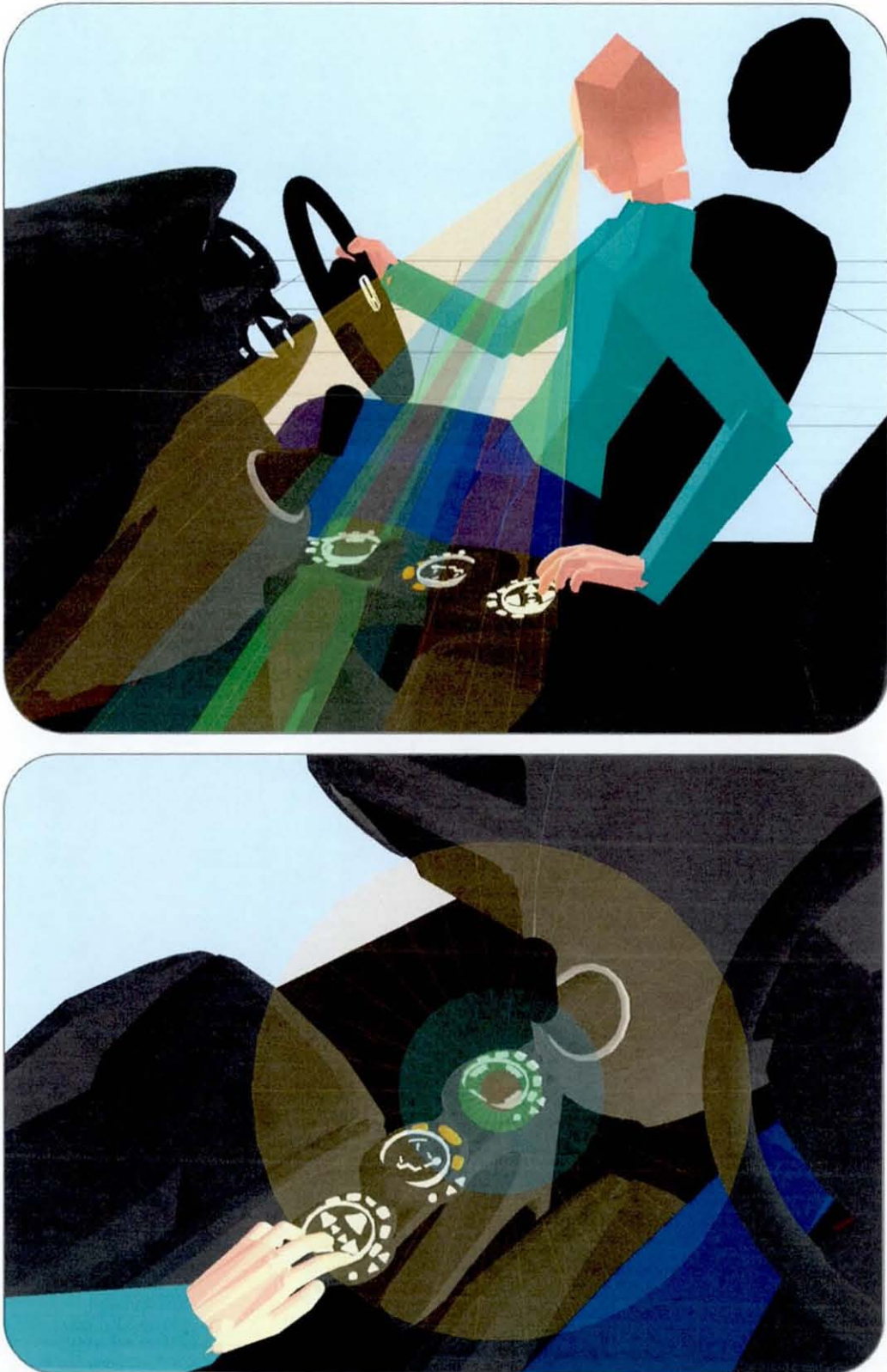
Figure 5.29: The visibility of the PTI for the 5th%ile Japanese female human model using a combination of comfortable head, neck and eye movement
