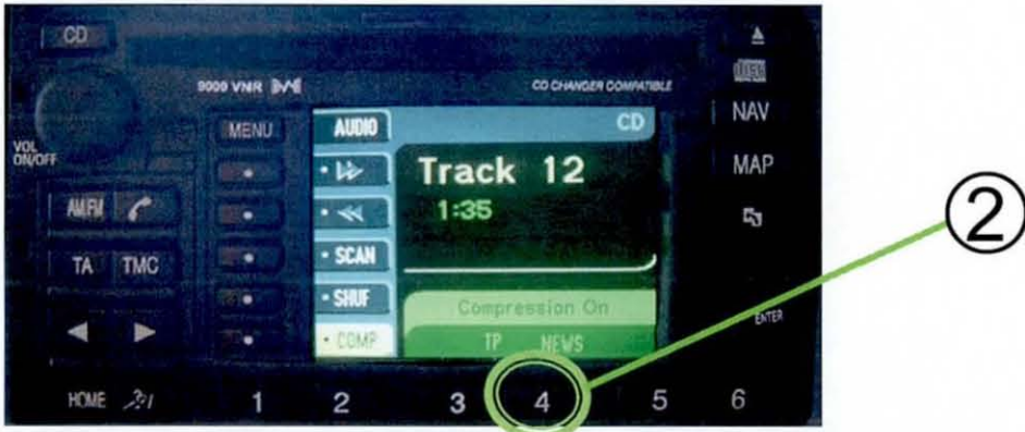
Figure 7.29. The task stages used to select a preset radio station on the baseline interface
