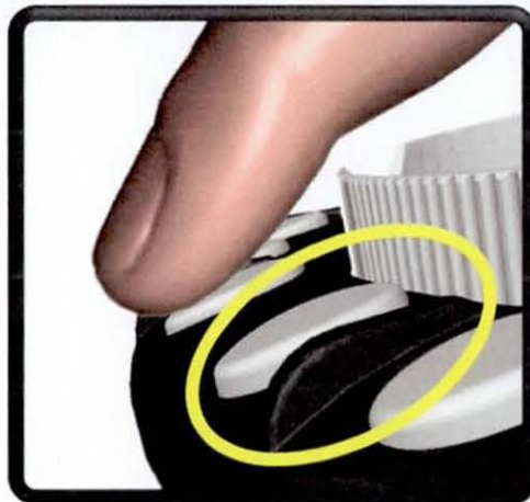
Figure 8.11. The 5mm high dividers used to separate groups of two preset buttons
