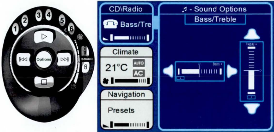
Figure 5.57. The screen shown on the second depression of the OPTIONS button Figure 5.57 shows the screen that is displayed on the second depression of the Options button. This screen allows for the control of Bass and Treble sound options. The skip forward and skip back buttons are used to vary the bass, and the play, stop buttons are used to vary the treble. The third depression of the Options button returns the main screen.
