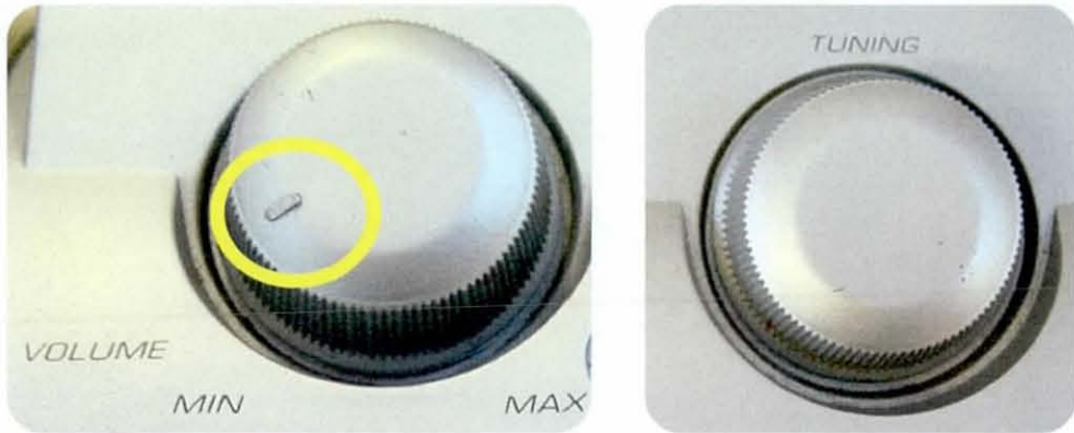
Figure 3.15. The rotary control that was used to change the volume, and the same shaped and sized radio tuning control
