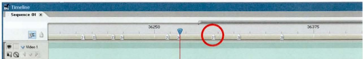
Figure 6.9. The timeline interface in Adobe Premiere Pro Version 7. The red circle highlights the marker system that was used to define the start and end of any glance that was performed during a task
