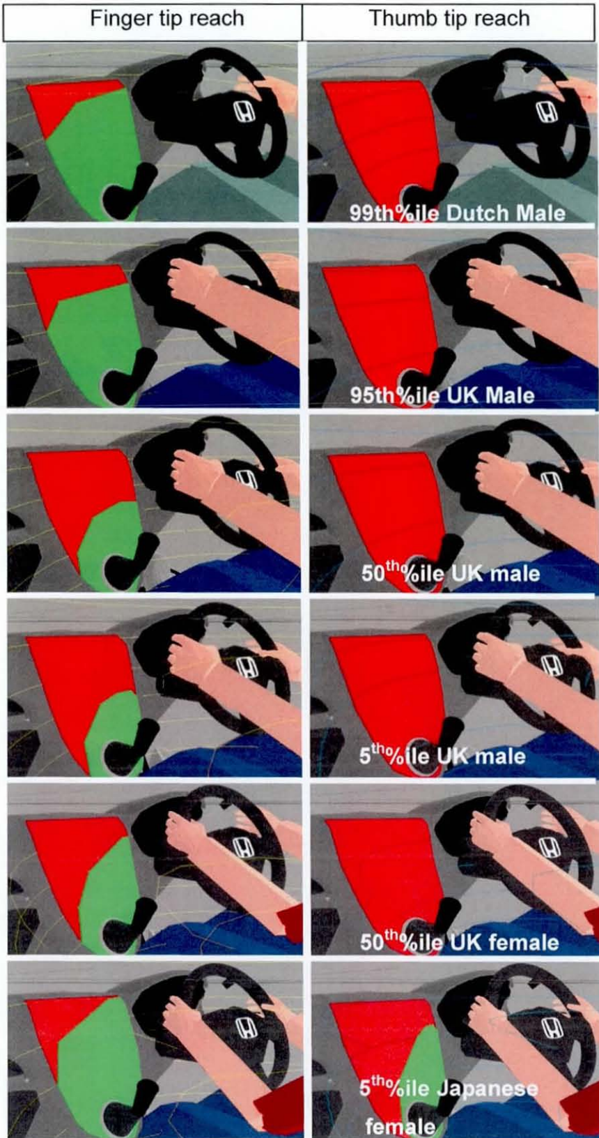
Fig 4.14: The results of the reach test performed for each human model reaching to the control panel with finger tip reach and thumb tip reach. The green areas show reachable surfaces, the red areas show the panel sections that are out of reach.
