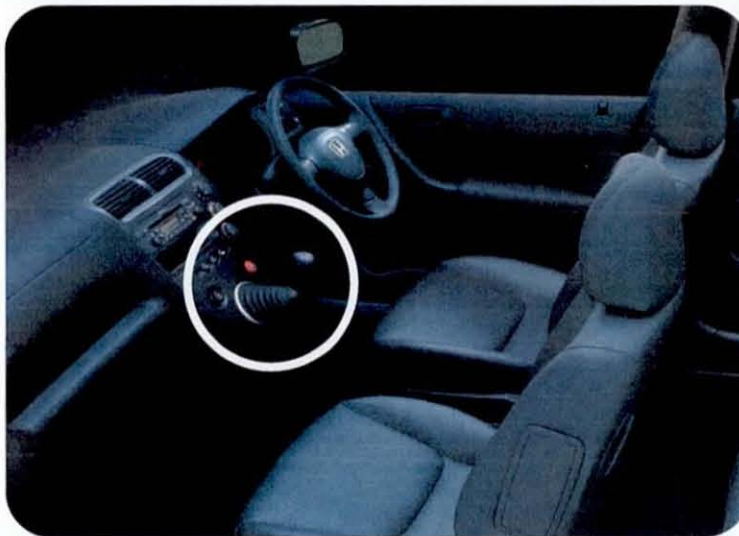
Figure 8.2. The interior of the 2001 Honda Civic, showing the unusual gear stick location that occupies the 'hot zone' for reach in the vehicle.
