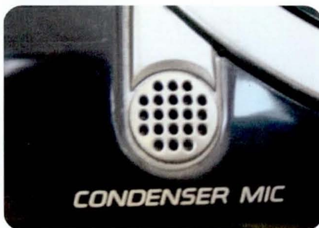
Figure 4.1. A microphone grille that was often mistaken for the eject CD button
