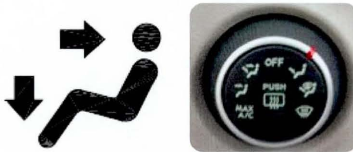
Figure 5.7: The standard airflow direction symbol that represents airflow to the face and feet BS ISO 2575:2004 and its implementation in a car control design
