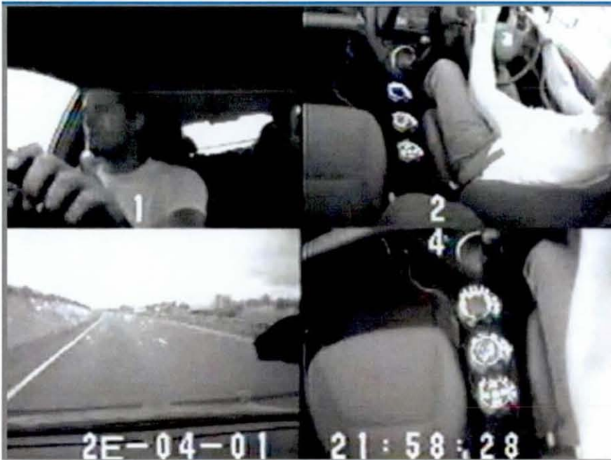
Figure 6.6. The view of the PTI system provided by the four lipstick cameras mounted in the Honda Civic
