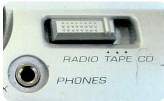
Figure 3.12. The slider switch used to select from the three modes of the portable HIFI
