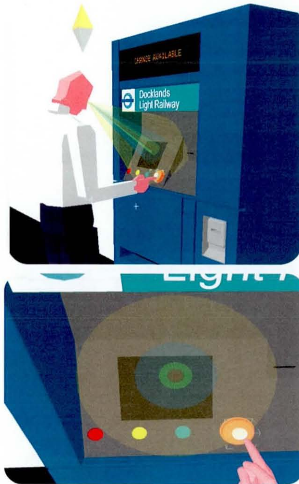
Figure 4.9: The use of the human's view function to assess the exact area that can be seen by the human model
