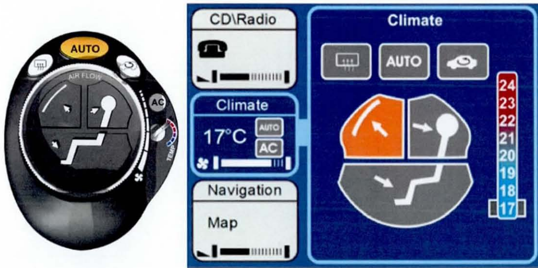
Figure 5.54. The HVAC PTI array and the associated software screen. The coloured circles show the button on the array and the associated on screen display
