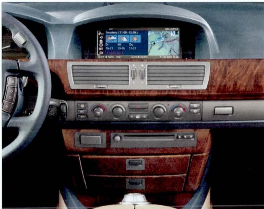
Figure 2.1. An example of a GUI in the automotive environment. The 2001 model BMW 7 Series with the I-Drive system
