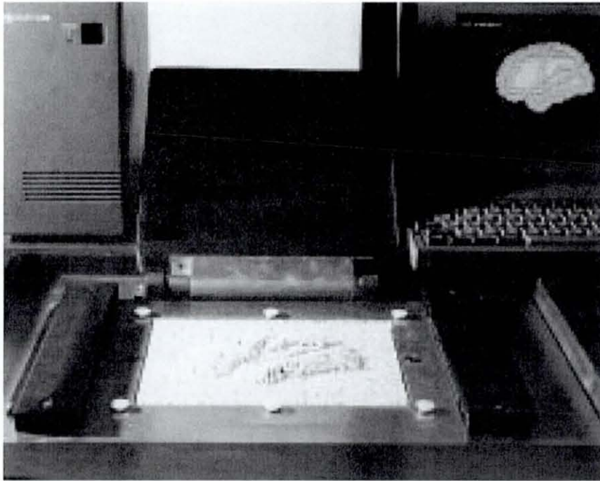
Figure 2.5. A 3D pin matrix display that is used to present tactile symbols and diagrams to blind people. Shinohara (1998)
