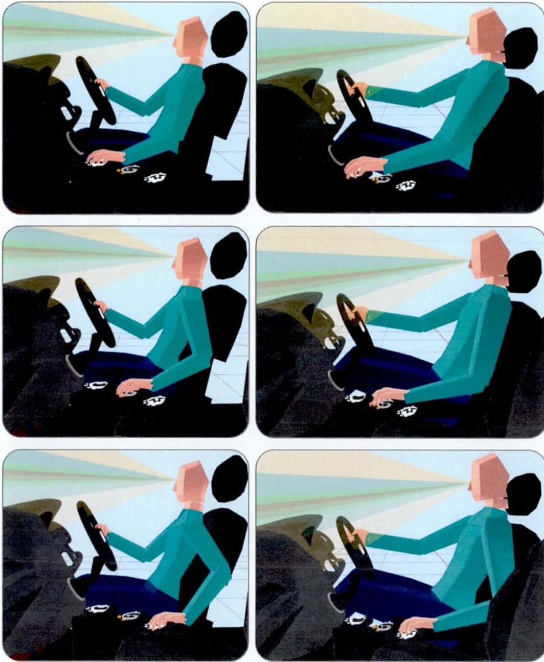
5.28. A reach test to determine the suitability of the angled design for the full range of users in the Honda Civic (left column, the 5 th %ile Japanese female, the right column the 95 th US male)
