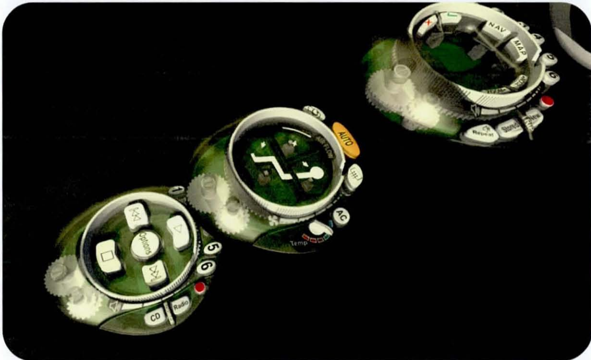
Figure 5.49. CAD renderings of the final PTI produced before rapid prototyping. Transparency has been applied to the array surrounds to allow a view of the internal structure in the bottom image
