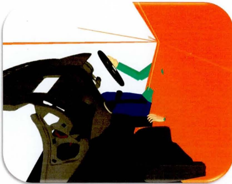
Figure 8.6. The hand, in the location required to access the ICE array, is shown to be in front of the contour that represents the limit of peripheral vision
