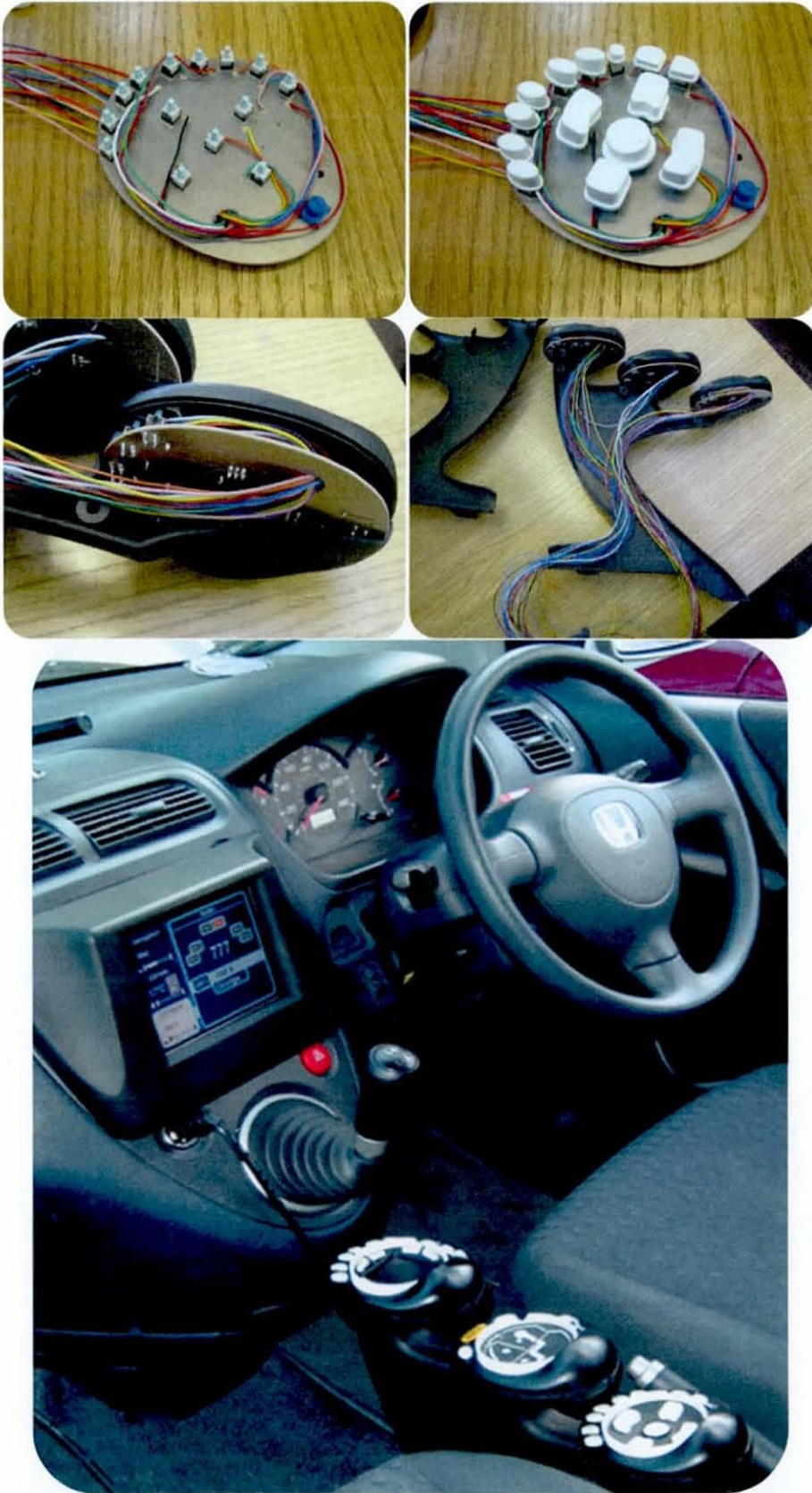
Figure 5.51. Assembly of the prototype parts (top four images). The final PTI interface in the 2001 Honda Civic, a full working prototype manufactured using rapid prototype technology
