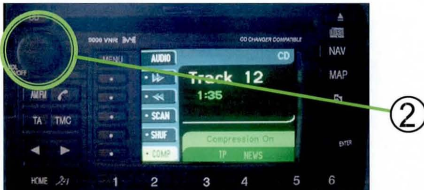
Figure 7.32. The task stages used to increase the volume on the baseline interface
