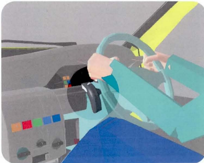
Figure 3.7: The multi modal concept 2. The device was located on the left hand side of the steering wheel. Functions would be selected via the white buttons
