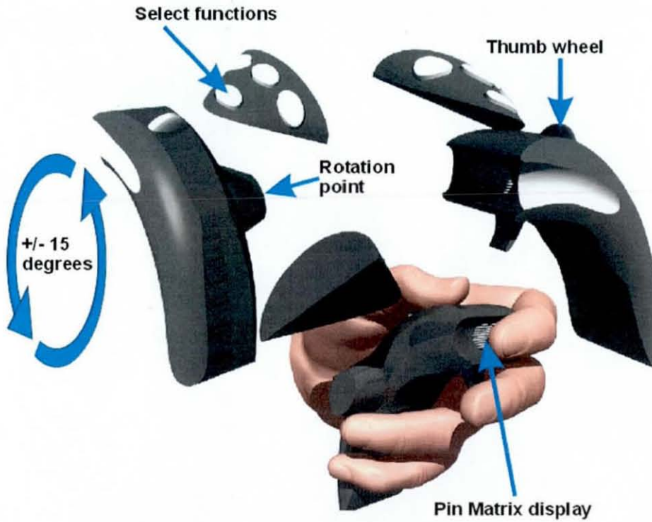
Figure 3.6: The multi modal concept 2. The device was located on the left hand side of the steering wheel 1. Functions would be selected via the white buttons
