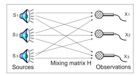
Figure 2.1. Diagram of instantaneous mixing with three sources and three measurements.
