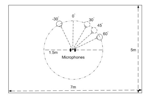
Figure 5.3. Plan view of the experiment setting in the room environment with two microphones and two sources
