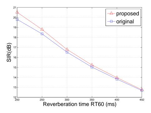
Figure 5.7. SIR comparison between original and proposed FastIVA algorithms as a function of reverberation time.
