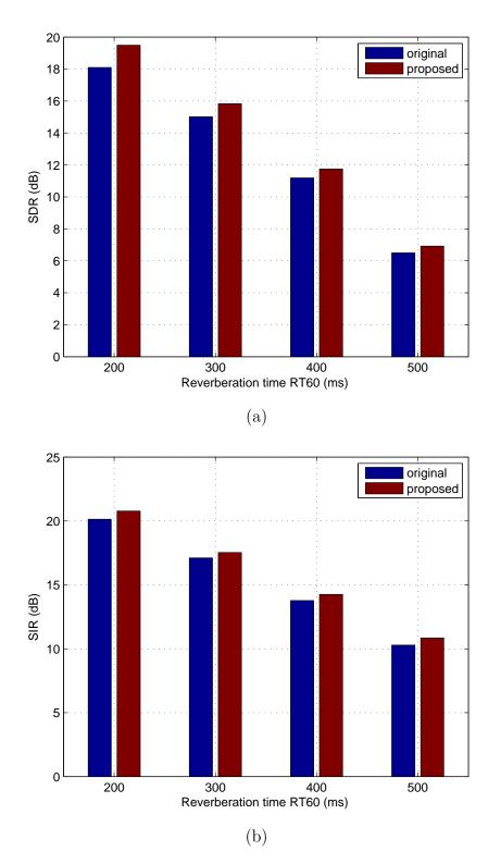
Figure 6.15. The separation performance in different reverberant environment for mixtures 4 (a) SDR (b) SIR
