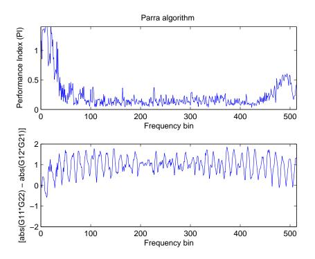
Figure 2.7. Separation performance of Parra's Method: performance index at each frequency bin for Parra's method at the top and evaluation of permutation at the bottom.
