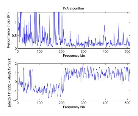
Figure 3.2. Separation performance by using original IVA.
