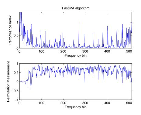
Figure 4.9. Separation performance of AVIVA in the noisy environment. The upper part is the performance index figure, and the bottom part is the permutation measurement figure.
