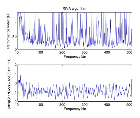
Figure 3.8. Separation performance by using robust IVA.
