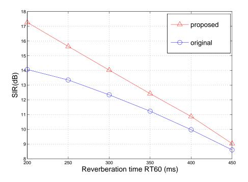
Figure 5.9. SIR comparison between original and proposed AuxIVA algorithms as a function of reverberation time.
