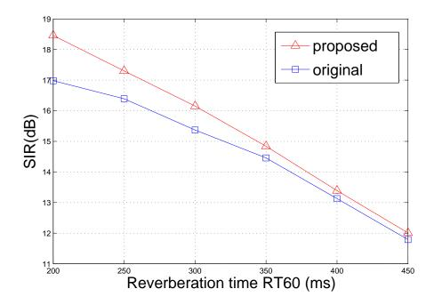
Figure 5.5. SIR comparison between original and proposed IVA algorithms as a function of reverberation time.
