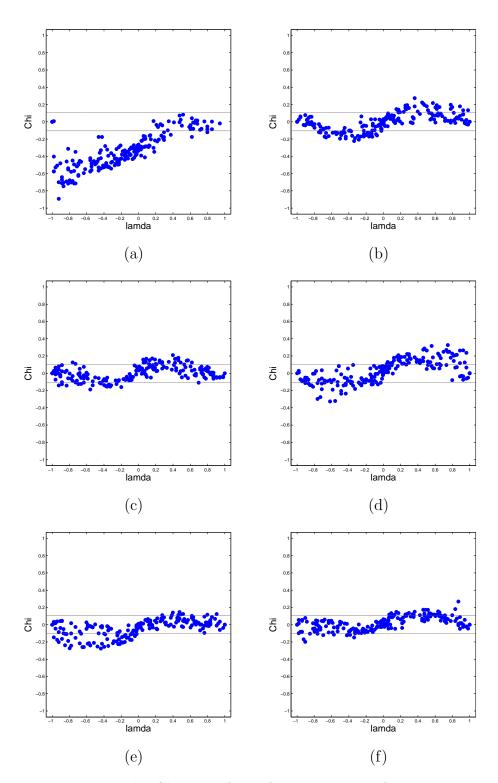
**Figure 6.10.** The Chi-plot of two frequency bins of a speech signal "sa1.wav" from TIMIT dataset (a) 50th and 51th frequency bins (b) 50th and 55th frequency bins (c) 50th and 60th frequency bins (d) 50th and 100th frequency bins (e) 50th and 200th frequency bins (b) 50th and 500th frequency bins
