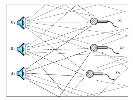
Figure 2.2. Diagram of convolutive mixing with three sources and three measurements.
