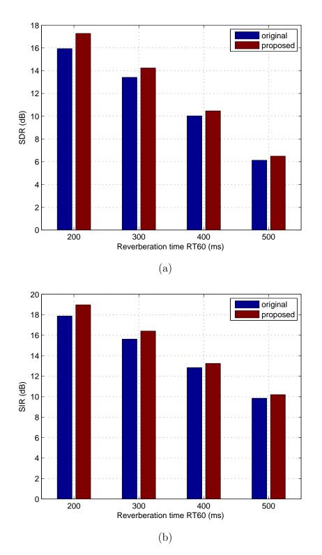
Figure 6.16. The separation performance in different reverberant environment for mixtures 5 (a) SDR (b) SIR
