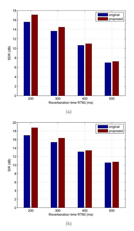
Figure 6.14. The separation performance in different reverberant environment for mixtures 3 (a) SDR (b) SIR
