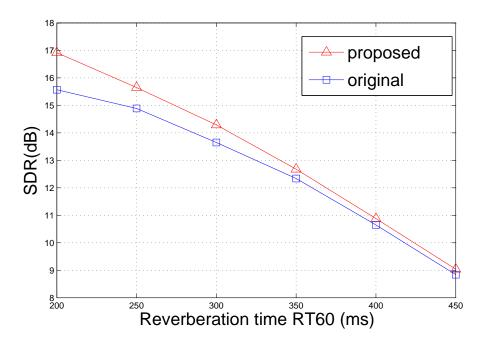
Figure 5.4. SDR comparison between original and proposed IVA algorithms as a function of reverberation time.
