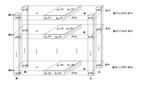
Figure 2.3. The mixture model of independent vector analysis. Independent component analysis is extended to a formulation with multidimensional variables, where the mixing process is constrained to the sources on the same horizontal layer.
