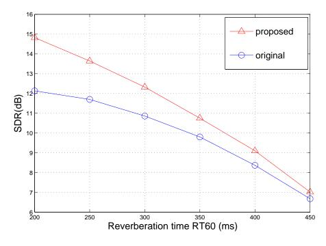
Figure 5.8. SDR comparison between original and proposed AuxIVA algorithms as a function of reverberation time.
