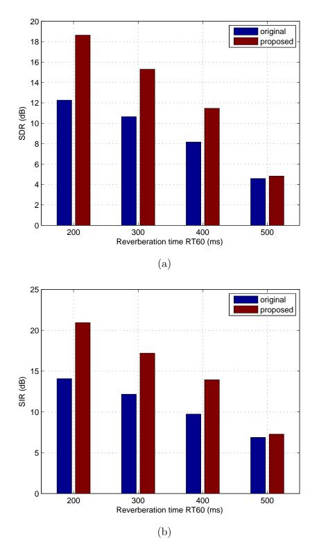
Figure 6.12. The separation performance in different reverberant environment for mixtures 1 (a) SDR (b) SIR
