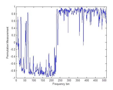
Figure 3.11. The permutation measurement showing the block permutation problem by using AuxIVA.
