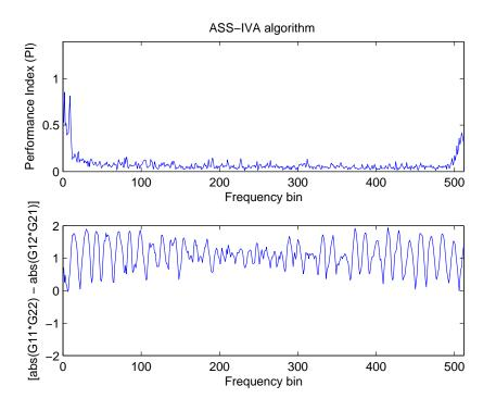
Figure 2.9. Separation performance of adaptive step size IVA method: performance index at each frequency bin for ASS-IVA method at the top and evaluation of permutation at the bottom.
