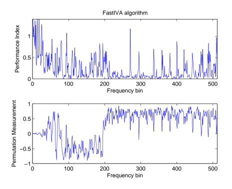
Figure 4.8. Separation performance of FastIVA in the noisy environment. The upper part is the performance index figure, and the bottom part is the permutation measurement figure.
