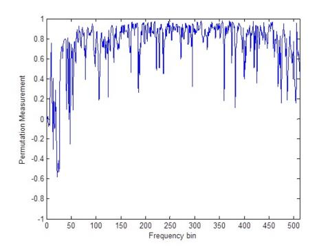
Figure 3.12. The permutation measurement without the block permutation problem by using AuxIVA with the proposed dependency model.
