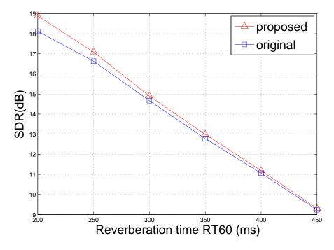
Figure 5.6. SDR comparison between original and proposed FastIVA algorithms as a function of reverberation time.
