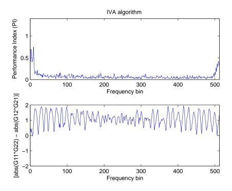
Figure 2.8. Separation performance of IVA method: performance index at each frequency bin for IVA method at the top and evaluation of permutation at the bottom.
