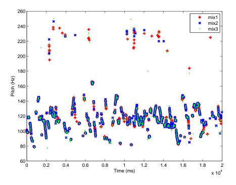
Figure 4.14. The pitch tracks of the mixed signals.
