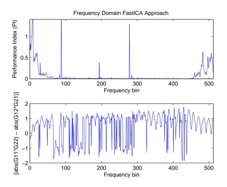
Figure 2.6. Separation performance of original FastICA Method: performance index at each frequency bin for the original FastICA method at the top and evaluation of permutation at the bottom.
