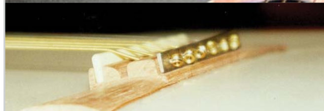
Undesirable distortion of soundboard under string tension
