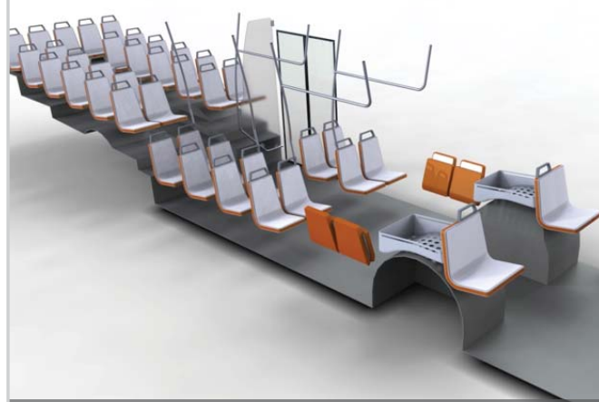
Modular components used to fit out the interior of a conventional rigid route bus to an existing customer specification – number of seats and layout thereof
