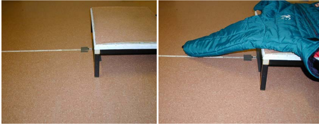
Figure 2. Photographs to illustrate platform and tape measure used for stiffness measurements and their positions during measurements of the drape of the sleeve of a garment.
