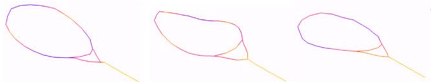
Fig.8. Example mode shapes for a hand-gripped racket left to right: B1, T1 and S1
