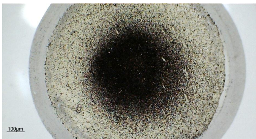
Figure 3.17: An image of the micro-particle sprayed on an agarose gel
