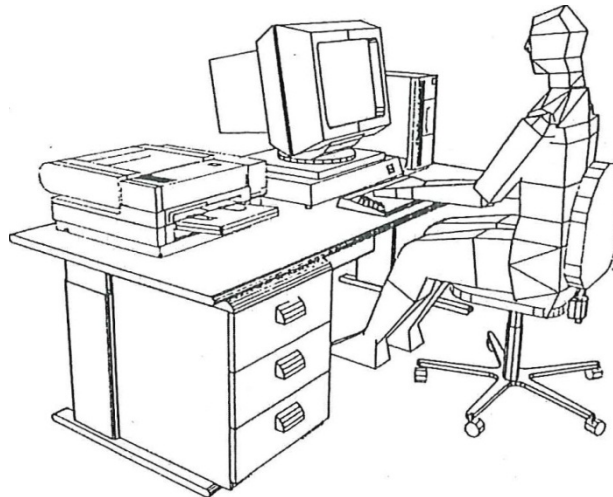
Figure 20.15. SAMMIE. An adjustable computer workstation model
