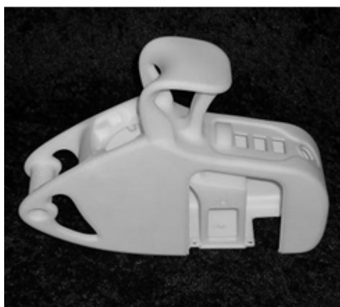
Figure 2. Single component tractor control pod casing (Burton, 2005).
