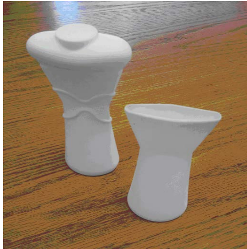
Figure 2. First prototype made from laser sintered polyamide
