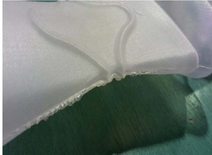
Figure 6. Unwanted “blow holes” along the bottle split plane.
