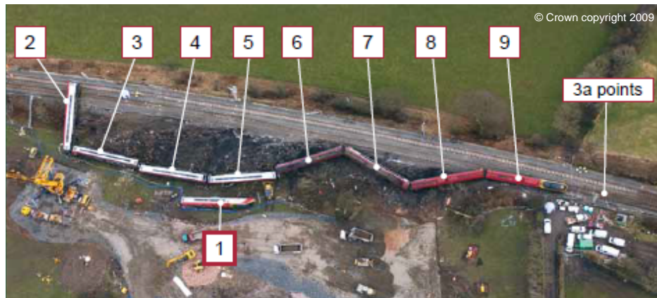
Figure 26 - Aerial view of the derailed train (numbers represent train vehicle number). From RAIB (2011).
