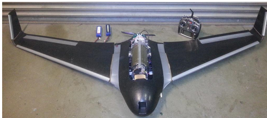
Figure 4. 2m wingspan X-8 Aircraft featuring mSOFC system, controller and hybrid batteries.
