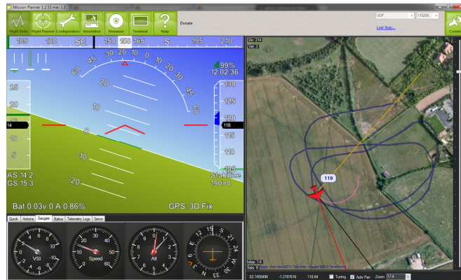
Figure 3. Real time telemetry and path plotting results
