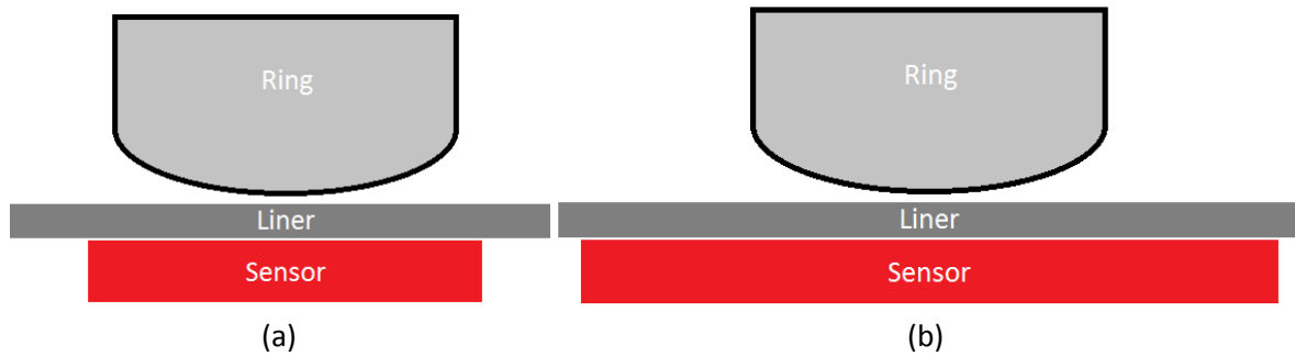
Figure 6.13: Representation of the sensor size for both sets of film thickness results. A sensor width approximately 10% larger than the ring's width (a) allows for reasonable deconvolution results, whereas double the ring's width (b) reduces the reliability of these results.
