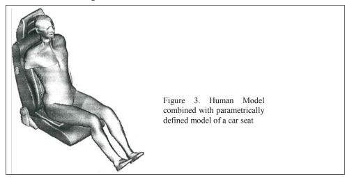
The investigation of deformations at the seat/human body interface had the objectives of determining variability in location of important design points (principally the eyepoint and the H-point) as drivers of different size and weight sit on seats with variable seat cushion compressibility, and the production of pressure distribution maps.
