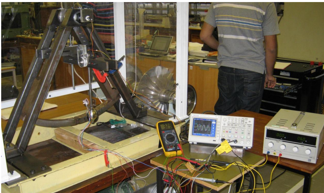
Figure 3.5.2n. Test rig with equipment and electrical test circuit set up for the gyro sensor tests
