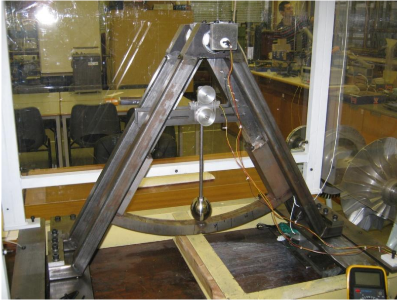
Figure 3.5.2a. Bell clapper test rig in its original form
