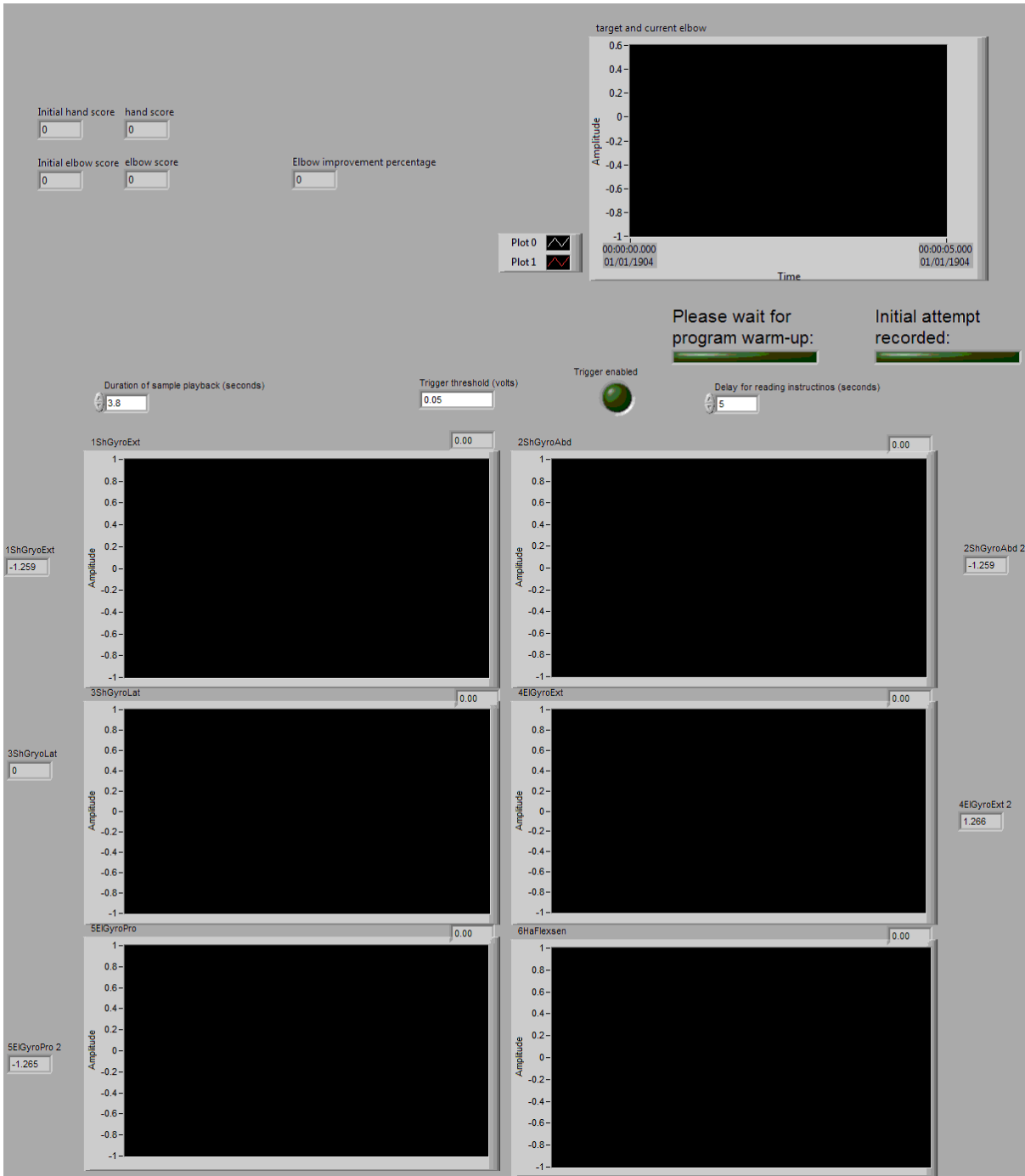
Figure 3.6.4c. Analysis area of the front panel of the feedback program showing a graphical display of the patient's elbow extension and flexion against the target movement and graphical displays of signals from all sensors during movements in the form of amplitude with time
