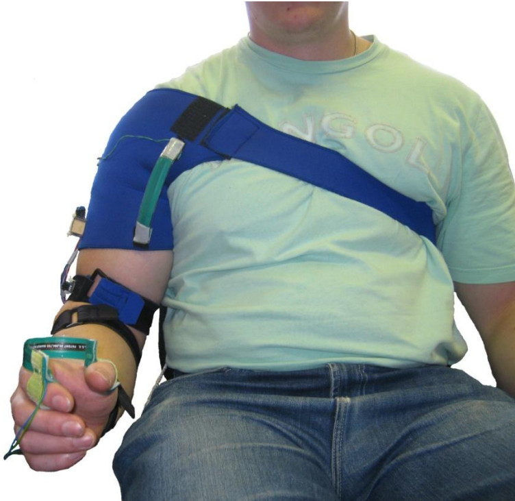
Figure 3.6.1d. Front view of the sensors and hardware of the prototype system
