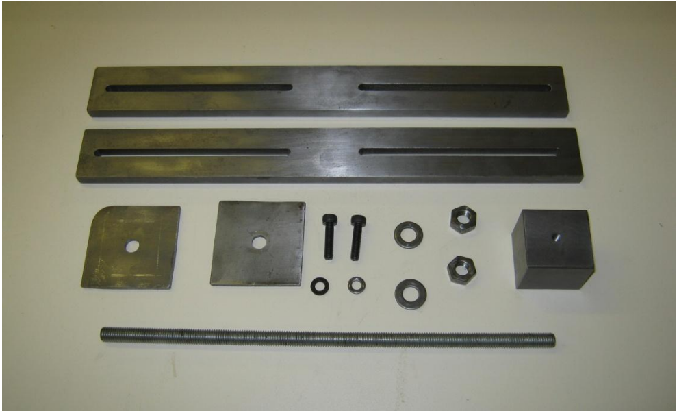
Figure 3.5.2b. Components constructed and sourced for modifications to the test rig
