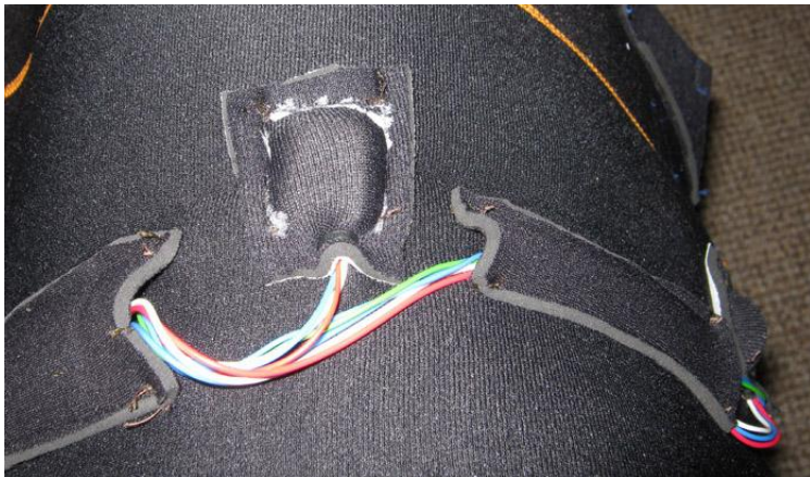
Figure 3.4.1f. A sensor mounted inside the sleeve with internal wiring shown
