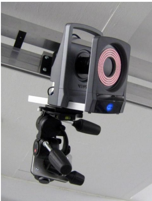
Figure 4.3.1b. A VICON camera with infrared LEDs and lens visible
