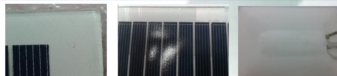
Fig. 3: Visual detection results with bubble near electrode (left), moisture ingress (middle) and edge/corner delamination (right)
