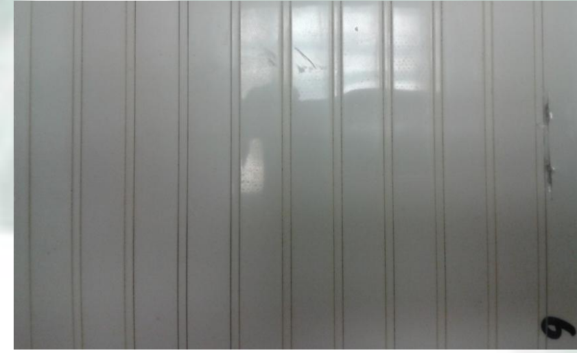
Fig. 1: Mini PV module after laser cutting. 100mm x 120mm, frameless P-Si
