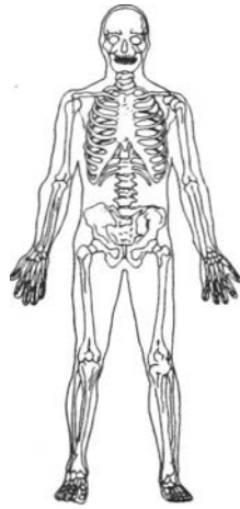
Figure 19.13. The link structure of the man model is a simplification of the human skeletal frame, with pin-joints suitably constrained to simulate human movement capabilities. The rigid links between the joint centres are defined by use of anthropometric data and are usually displayed with 3D flesh shapes.
