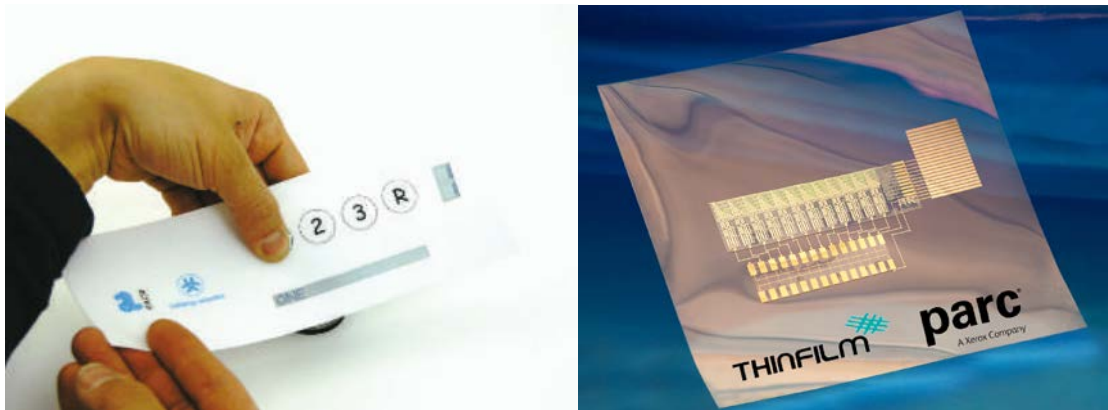
Figure 2-3 Printed electronic prototypes i (a) The system-on-a-sheet demonstrator developed by Linköping University and the Acreo Institute in Sweden 26 ii (b) Thinfilm's first scalable printed CMOS (complementary metal-oxide-semiconductor) memory 27
