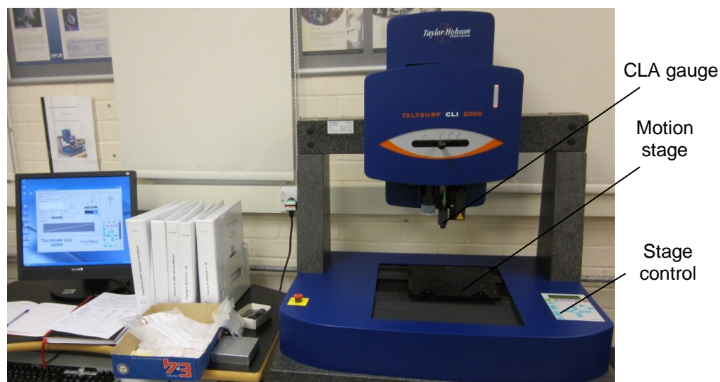
Figure 4-9 Talysurf CLI 2000 with a CLA gauge
