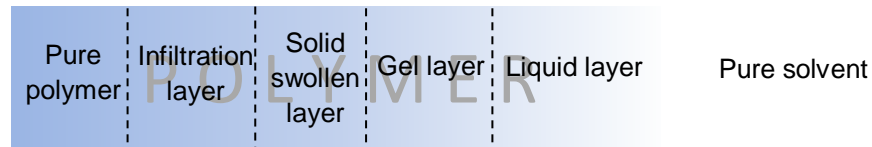
Figure 5-13 Illustration of different layers in polymer dissolved in a solvent. Separation between different layers is imaginary, and there is no marked border between layers in practice.
