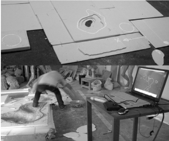
Figure 8 : Negative foam mould before and after addition of fibre-reinforced plaster
