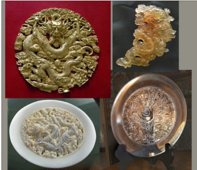
Figure 3.4a Examples of product effects produced by 3D scanning, data manipulation and AM
