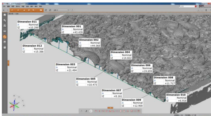
Figure 3.1c Measuring on any sectional view
