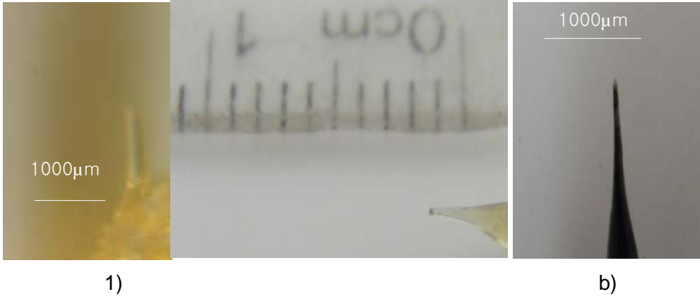
Figure 3 digital image of microneedles fabricated from fish scale a) Plain and b) containing methylene blue
