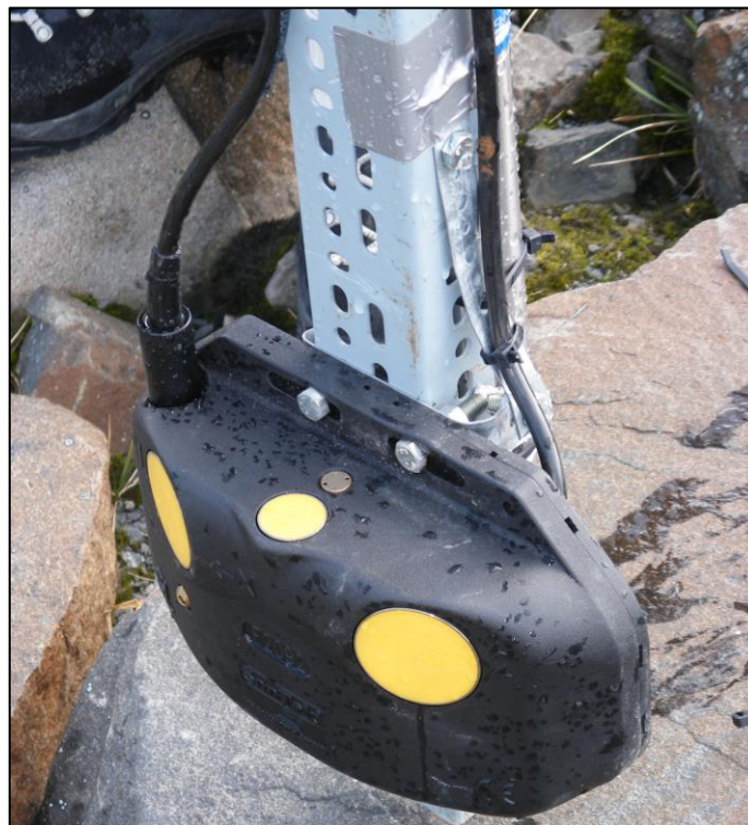
Figure 3.3. Photograph of a SonTek/YSI Argonaut-SL prior to deployment at Nordjåkk. Model shown is the SL1500.
