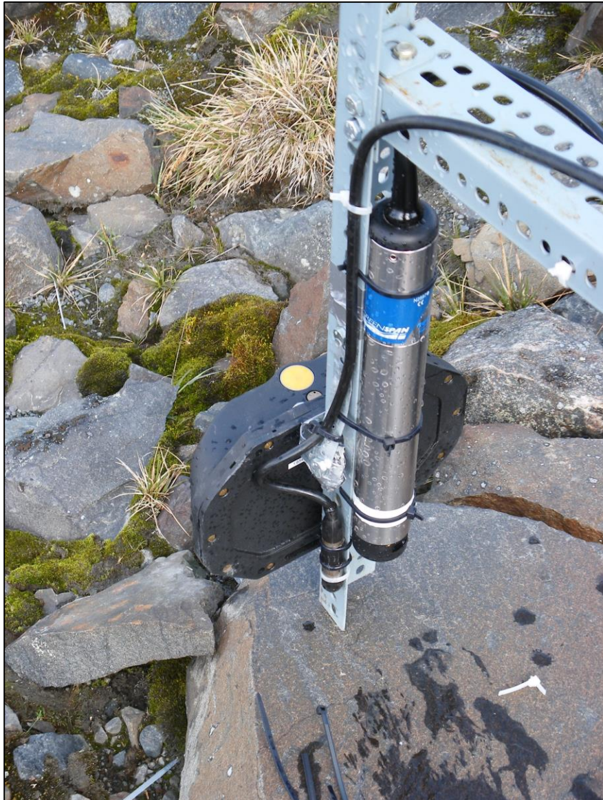
Figure 4.1. Photograph of the Greenspan TS100 turbidity probe prior to deployment at the Sydjàkk gauging station
