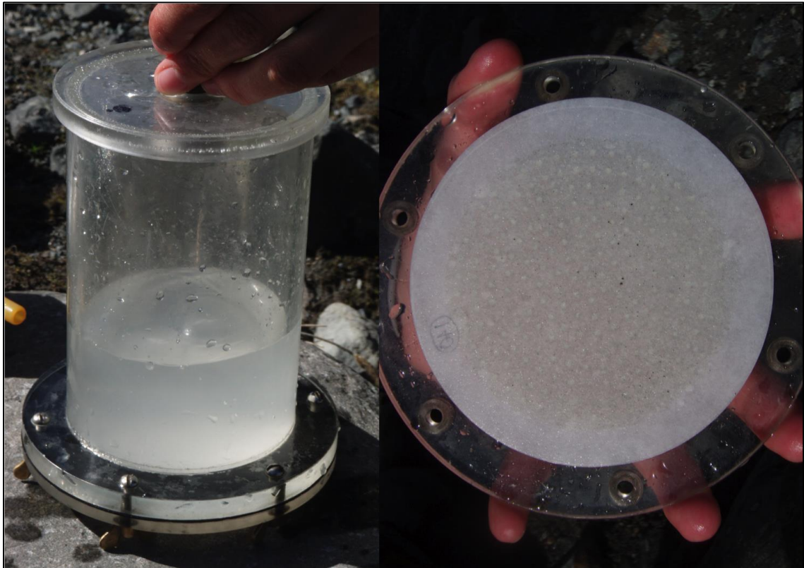
Figure 4.2. Photographs of the filtration apparatus used in the study (left), and a Whatman-Grade 40 filter paper following sample filtration (right)
