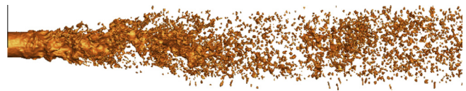
Fig. 35. LES of liquid jet primary breakup on mesh II. U_l = 4 m/s, U_c = 166 m/s.
