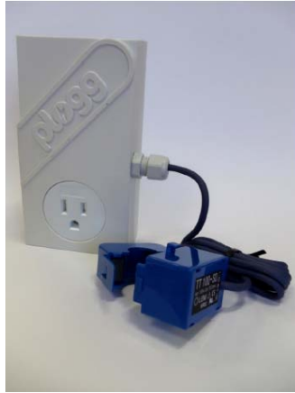
Figure 4-3 Current clamp logger: Plogg with external 100 Amp current transformer (Energy Optimizers 2010)
