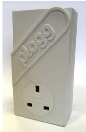
Figure 4-5 Plogg Smart Meter Plug (Energy Optimizers 2010)
