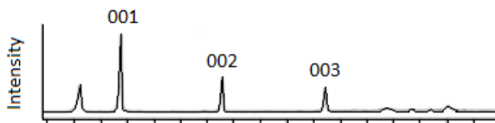
Figure 9: Simple diagram of LDH reflections which align in a plane to give much stronger reflections than would otherwise be observed.
