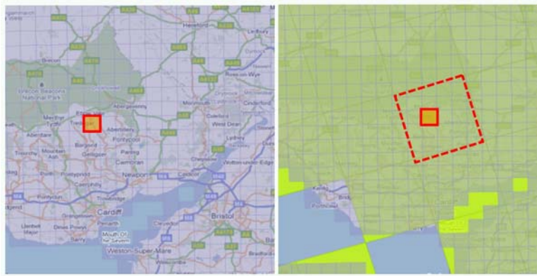
Figure 4 Showing UKCP09 5km and 25km grid resolutions for South Wales/ Severn region
