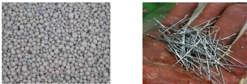
Figure 2.4 Sintered Pulverised Fly Ash (SPFA) Aggregate and Maccaferri FF3 Wirand Steel Fibres
