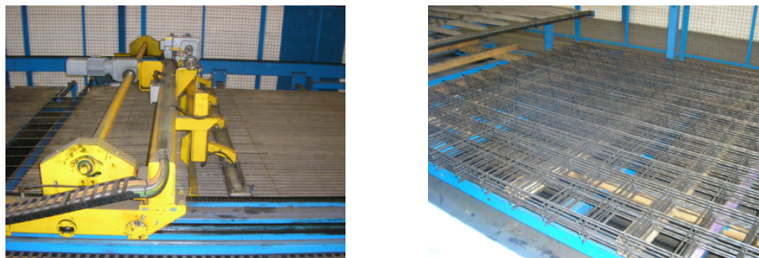
Figure 1.3 Automated Welded Mesh Manufacture at Hanson Manufacturing Facility, Hoveringham
