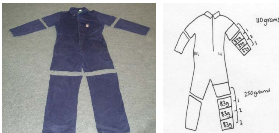
Figure 2.3. Photograph of cut-up overall to determine weight distribution of garment weight and diagram to illustrate methodology of calculating weight corrections applied using wrist and ankle weights.
