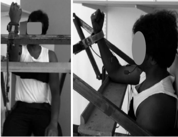
Figure 6.1 The isometric strength testing apparatus used to measure elbow flexion/extension force.
