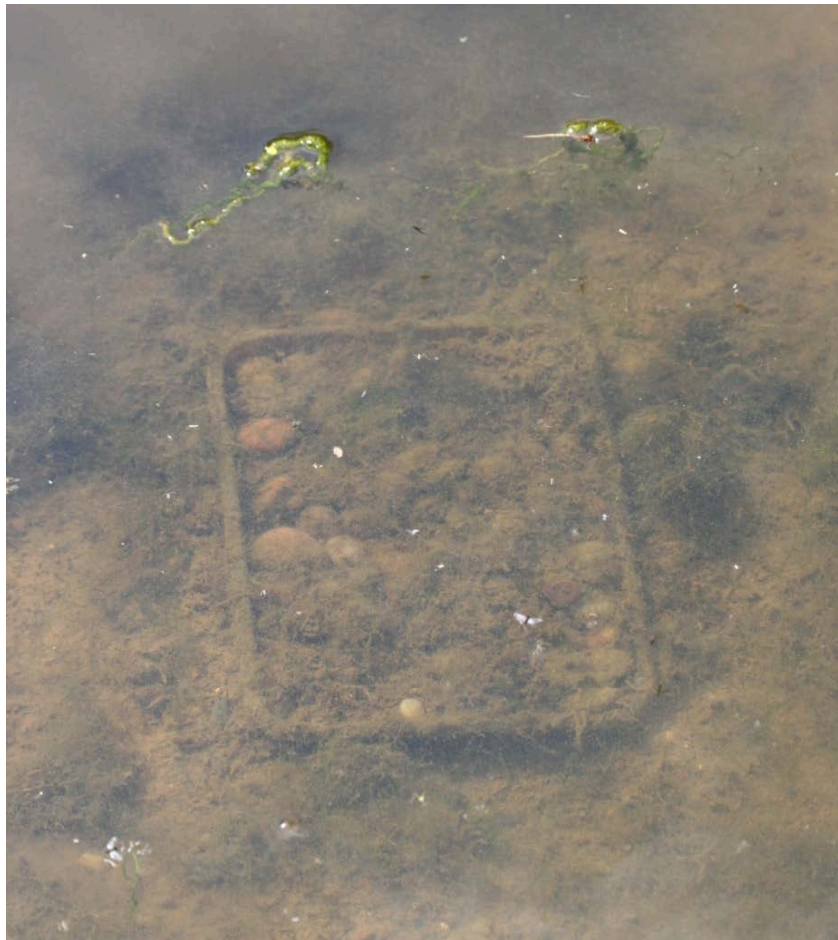
Plate 4.5 A River Eye sediment trap in-situ after being in the river for a period of 21 days. This clearly shows sedimentation and excessive algal growth to be a significant problem within the river.
