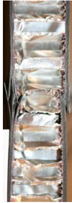
Fig.17. Photographs showing a side view of an impact-damaged sandwich panel after CAI test
