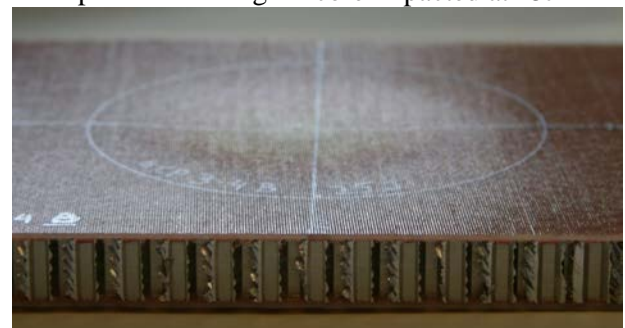
Fig.14. Impact damage in an 8/8 CP E-glass/epoxy panel with 70 \text{ kg/m}^3 core impacted at 25J
