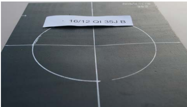
Fig.6. A 16/12 QI carbon/epoxy sandwich panel with 70\text{kg/m}^3 core impacted at 35J
