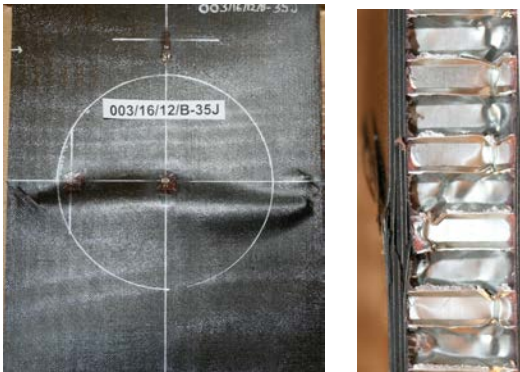
Fig.18. Photographs showing front and side view of an impact-damaged sandwich panel after CAI test
