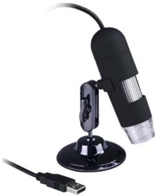
Fig.2. Hand held USB microscope used to capture damage propagation during compression test
