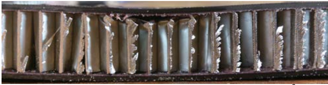
Fig.12. A 8/8 sandwich panel with 140 \text{ kg/m}^3 impacted at 25J
