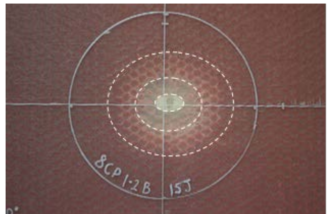
Fig.13. Impact damage in an 8/8 CP E-glass/epoxy panel with 70 \text{ kg/m}^3 core impacted at 15J
