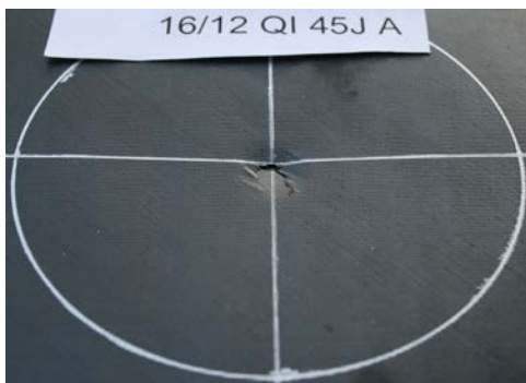
Fig.7. A 16/12 QI carbon/epoxy sandwich panel with 70\text{kg/m}^3 core impacted at 45J
