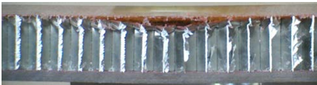
Fig.16. A 16/16 E-glass/epoxy sandwich panel impacted at 18J
